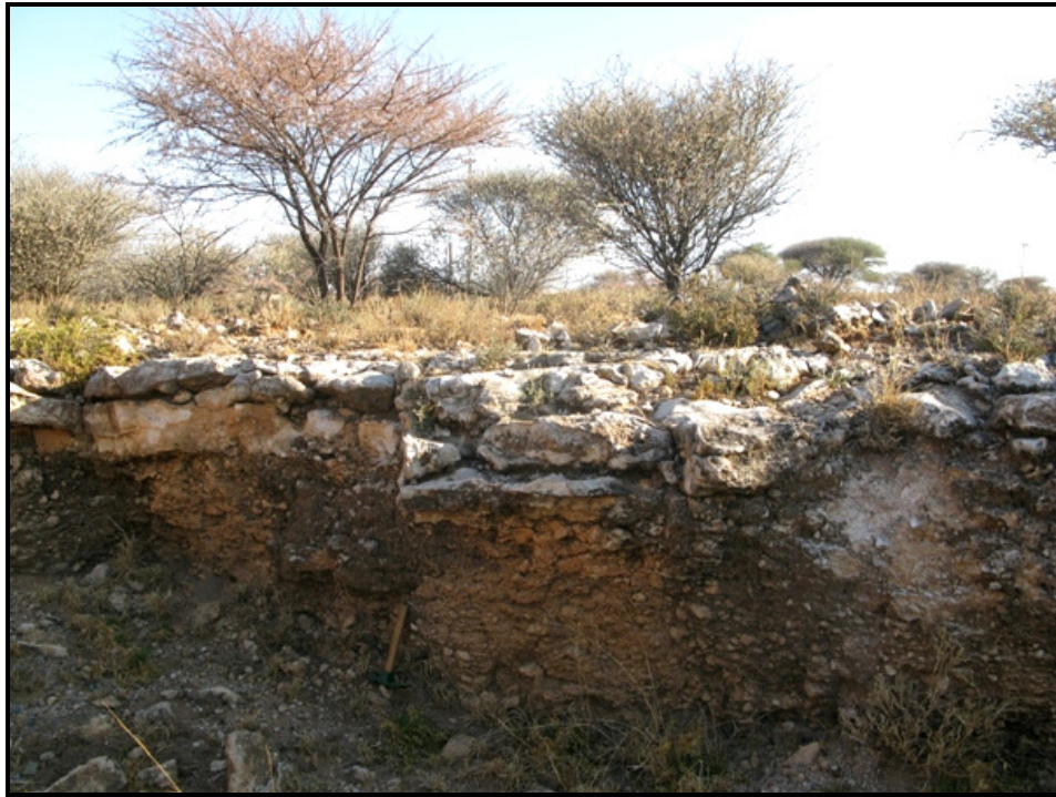
Fig. 21. Thick, nodular calcrete overlain by well-consolidated calcrete hardbank in a borrow pit just SE of the Herbert substation (Hammer = 27cm) (Loc. 608).
