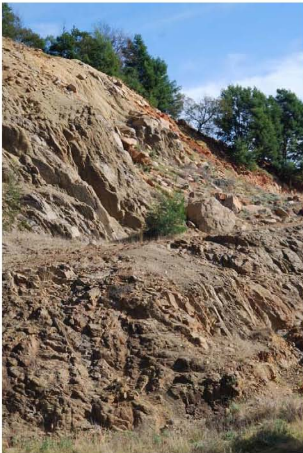
Figure 3: Borrow pits 2 (above) and 5 (below) showing deeply weathered and fresher dolerite respectively. The route followed by the road itself does pass a number of roadcuttings containing buff to maroon mudstones of the Burgersdorp Formation. These are situated immediately north of the
