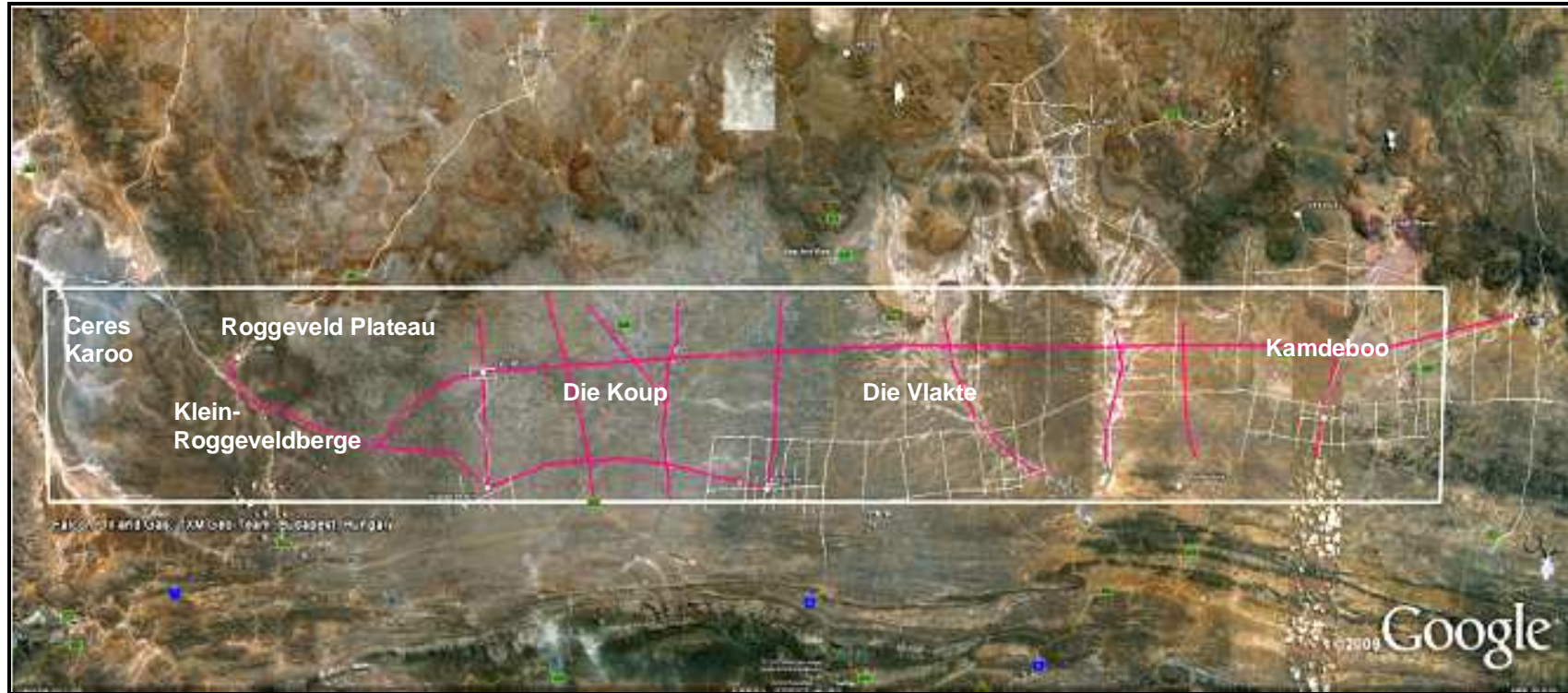
Fig. 2. Satellite image of the Great Karoo region sensu stricto , stretching between the Cape Fold Mountains in the south and the Great Escarpment in the north (Image kindly provided by SRK Consulting). The TCP prospecting area is outlined by the white rectangle. The approximate alignments of the proposed new seismic survey corridors are indicated by pink lines.
