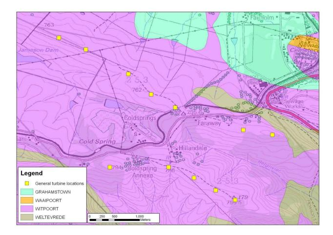
Fig. 1: Geological map of Waainek illustrating the position of the proposed wind turbines
