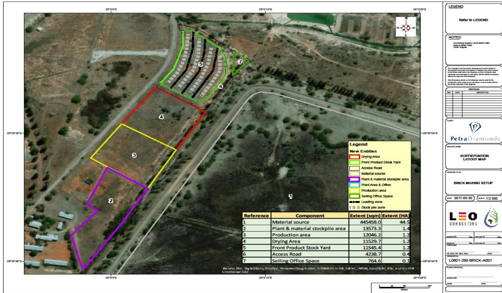
Figure 4. Layout of the various infrastructural components of the proposed brick-making plant, Koffiefontein diamond mine (Image supplied by Greenrsa (Pty) Ltd).
