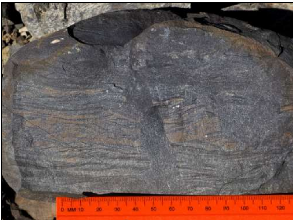
Figure 48. Vertical section through a ripple cross-laminated sandstone bed showing the subvertical cast of a plant stem / root or fossil burrow (Loc. 567) (Scale in cm and mm).
