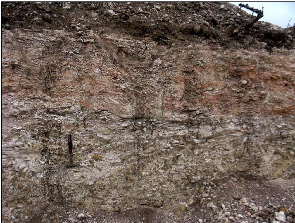
Figure 15. Calcretised conglomerates and grey to pinkish calcareous aeolianites of the Alexandria Formation exposed in a borrow pit cut face, Steins Valley 202 (Loc. 184) (Hammer = 30 cm). This borrow pit is not part of the wind farm project.
