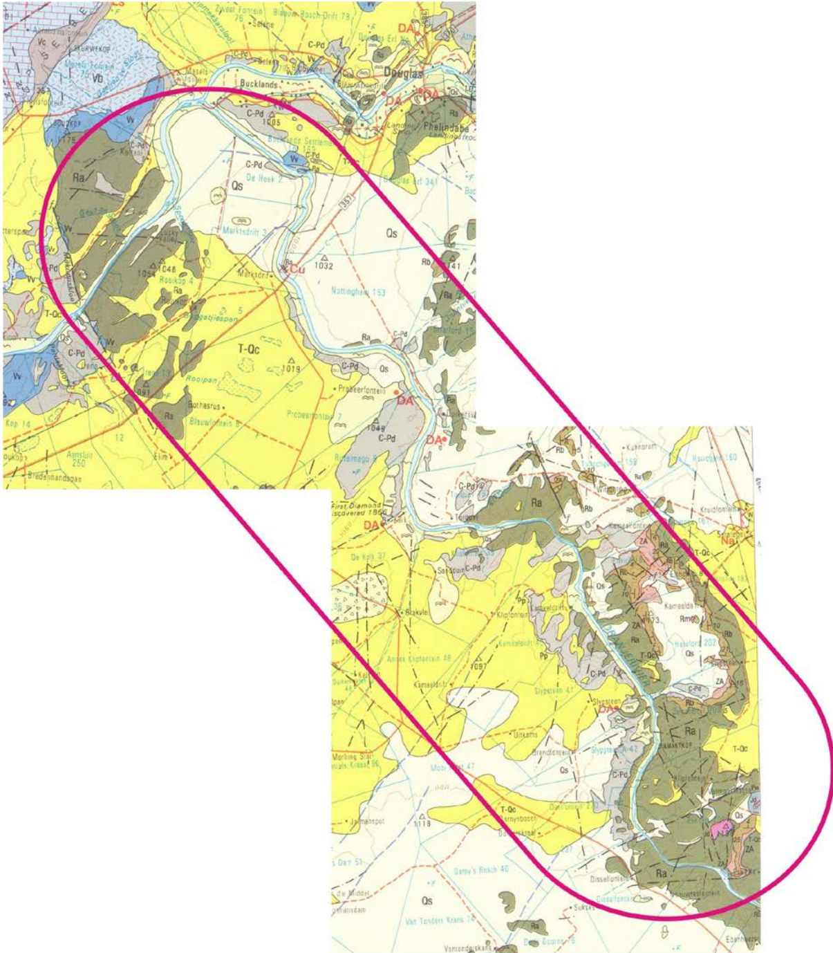
Figure 2. Portion of 1: 250 000 geological map 2922 Prieska (Council for Geoscience, Pretoria) showing approximate location of the proposed hydroelectric facility 26 km south of Douglas. The study areas are underlain at depth by Precambrian lavas of the Allanridge Formation (Ventersdorp Group, Ra ) as well as Dwyka tillites (Mbizane Formation, C-Pd ) and basal Ecca mudrocks (Prince Albert Formation, Pp ) of the Karoo Supergroup. The basement lavas and Karoo sediments are largely overlain by Late Cenozoic superficial deposits made up of cf. Plio-Pleistocene or older terrace gravels, aeolian sands ( T-Qc , Qs ) and geologically recent alluvium.
