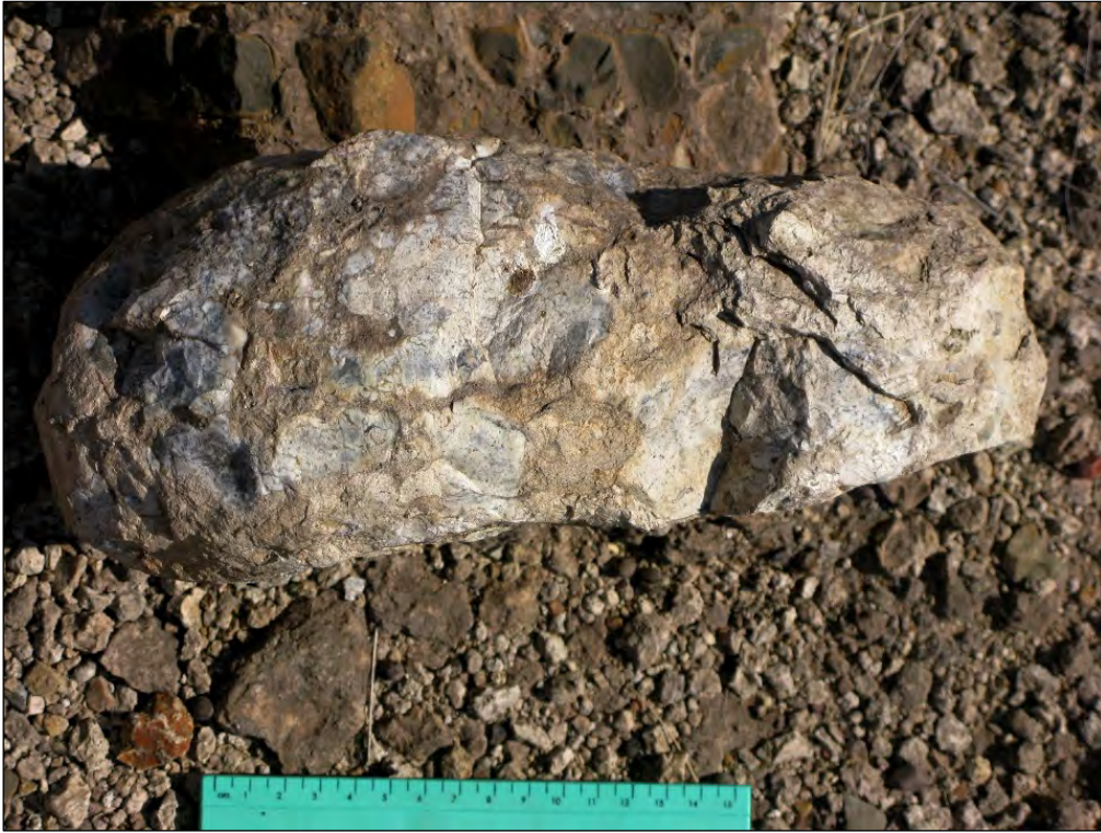
Fig. 50. Elongate, cobble-sized cherty concretion weathered out from the basal silicified calcrete zone (Scale in cm).
