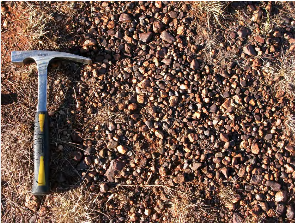
Fig. 69. Better rounded surface gravels and reddish sandy soils observed locally in Borrow Pit 1 study area, Postmasburg (Hammer = c. 30 cm).
