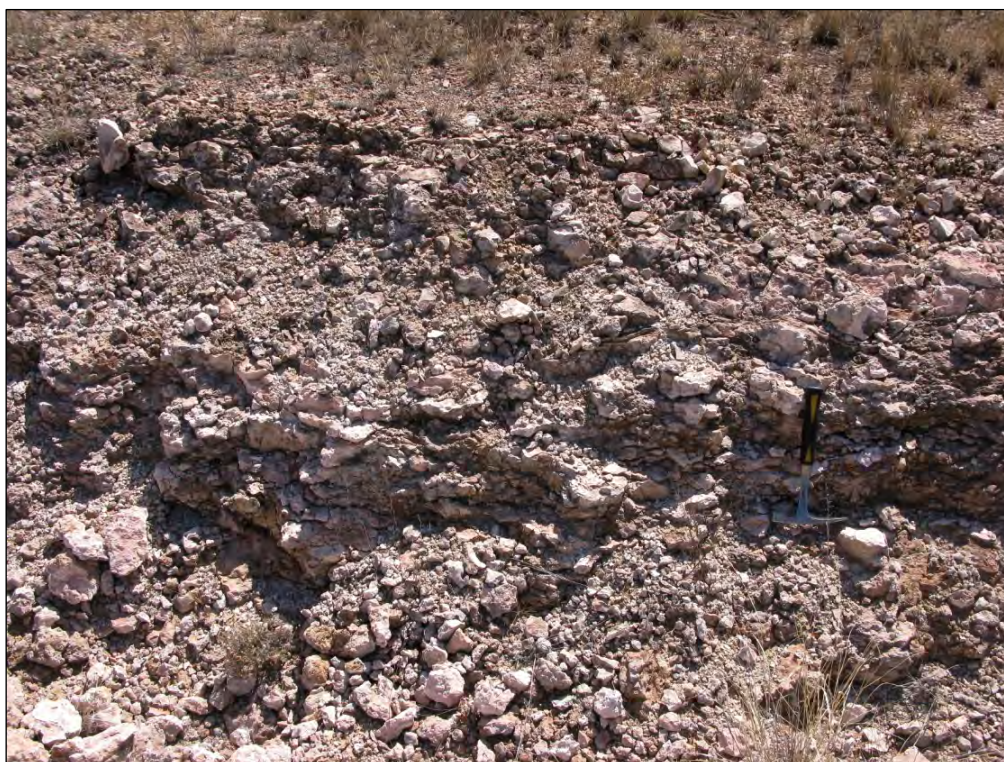
Fig. 70. Crudely bedded, rubbly surface calcrete exposed in an existing borrow pit just north of the proposed Borrow Pit 1 study area at Wincanton (Hammer = c. 30 cm).
