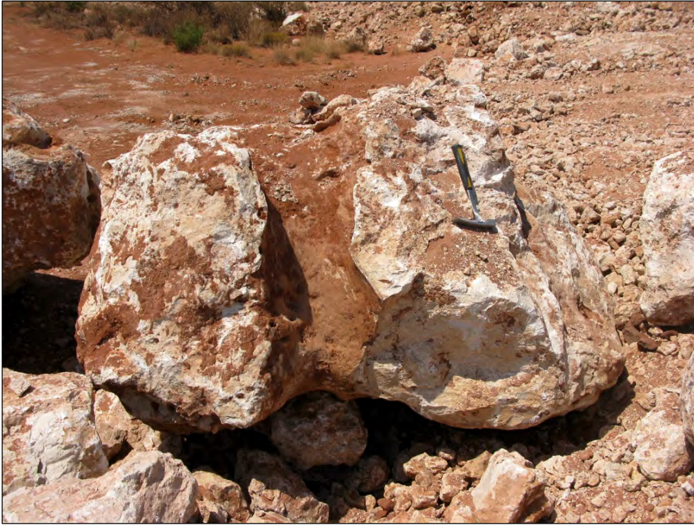
Fig. 43. Excavated block of surface calcrete showing large, subvertical silt-lined solution hollow, Sishen loop study area (Hammer = c. 30 cm).
