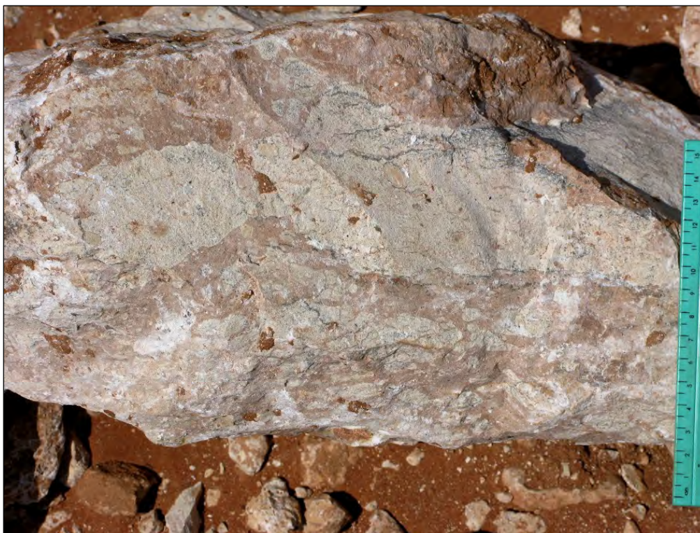
Fig. 42. Dense calcrete breccia, possibly formed by partial replacement and in situ brecciation of a silcrete horizon, Sishen loop study area (Scale in cm).
