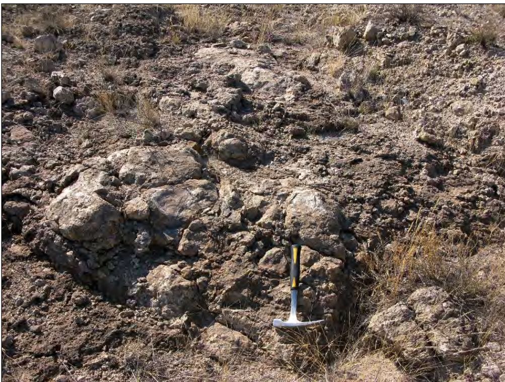
Fig. 49. Basal silicified calcrete in Borrow Pit 2 site showing irregular cherty concretions (Hammer = c. 30 cm).
