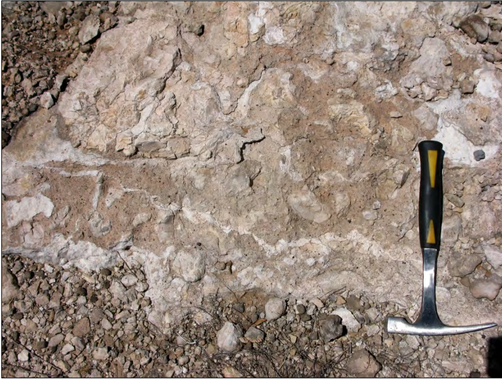
Fig. 58. Well-consolidated, reworked calcrete rubble within a pale brown, finely-gravelly matrix, Trewil Borrow Pit 2 study area (Hammer = c. 30 cm).
