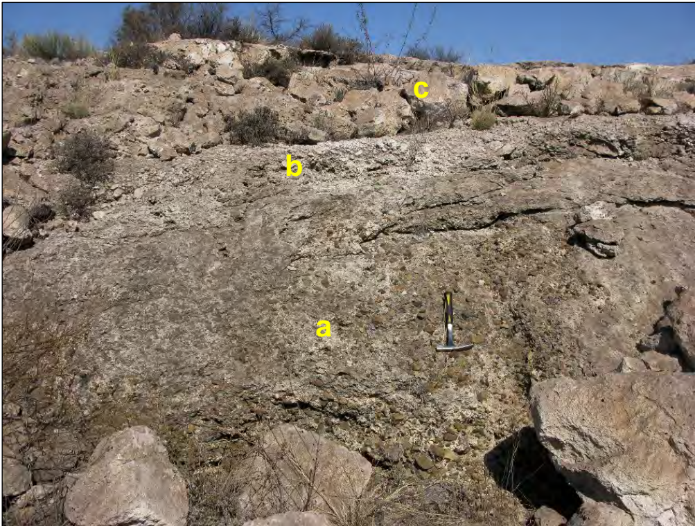
Fig. 48. Same locality as in previous figure, showing (a) poorly-sorted calcretised gravels infilling a palaeochannel; (b) thin horizon of rubbly calcrete; and (c) bioturbated calcrete hardpan (Hammer = c. 30 cm).
