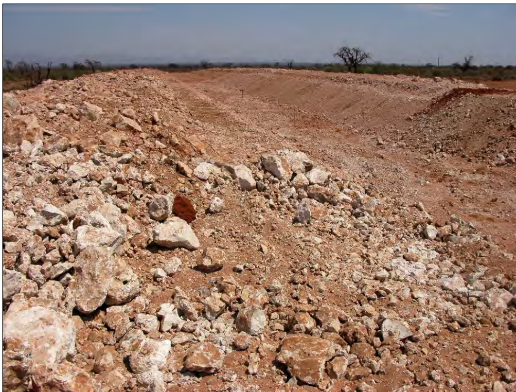
Fig. 41. Recently-excavated trench through thick surface calcretes in the Sishen loop study area.
