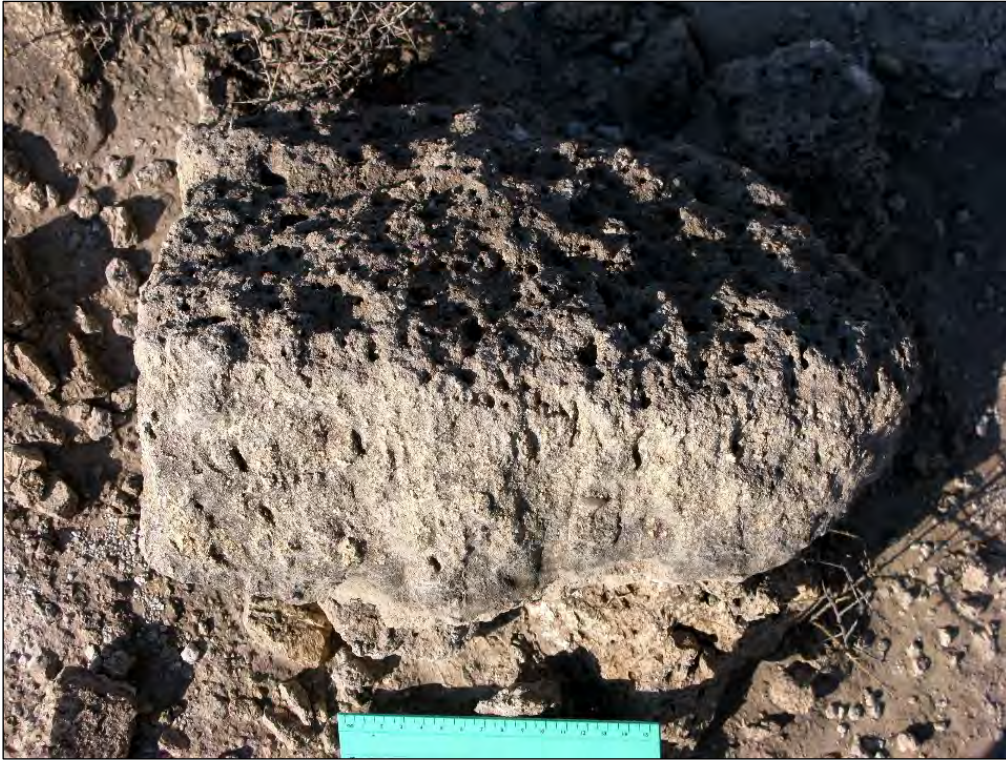
Fig. 73. Displaced block of impure, greyish sandy calcrete within the upper Kalahari succession at Witloop (Borrow Pit 1 study area) that is permeated by numerous narrow hollow tubes.
