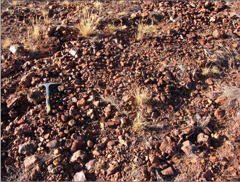
Fig. 68. Polymict mixed alluvial and colluvial surface gravels, test pit in Postmasburg Borrow Pit 2 study area (Hammer = c. 30 cm).
