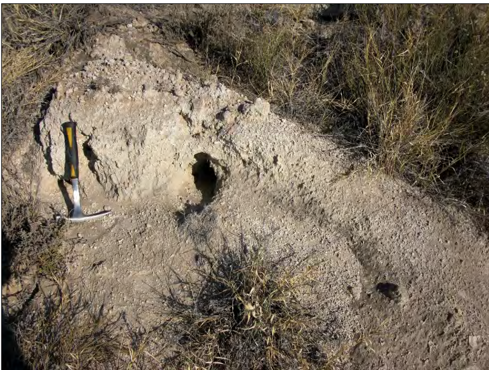
Fig. 74. In situ impure calcrete horizon riddled with fine calcrete tubules, seen weathering out from the profile here, Witloop Borrow Pit 1 study area (Hammer = c. 30 cm).
