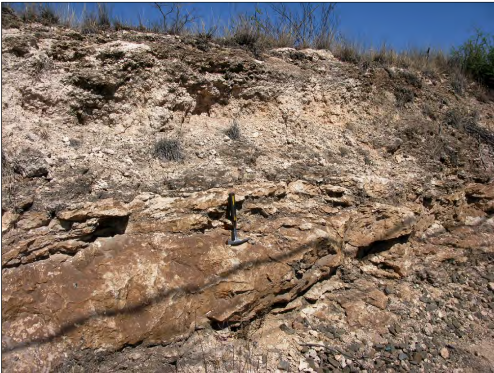
Fig. 22. Contrast between the lower, well-consolidated, brownish weathering (possibly manganese-stained) lower calcrete unit and the upper, crumbly calcrete with a hard hardpan capping, Ulco railway cutting (Hammer = c. 30 cm).
