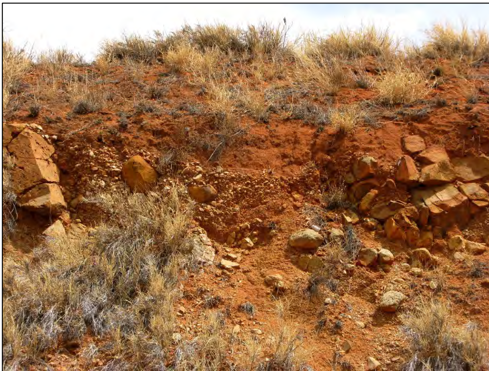
Fig. 9. Basement highs of blocky-jointed Ventersdorp Group andesites flanking a shallow gully infilled with mixed colluvial and alluvial gravels (note rounded corestones), the whole blanked beneath orange-brown Hutton sands, Fieldsview railway cutting
