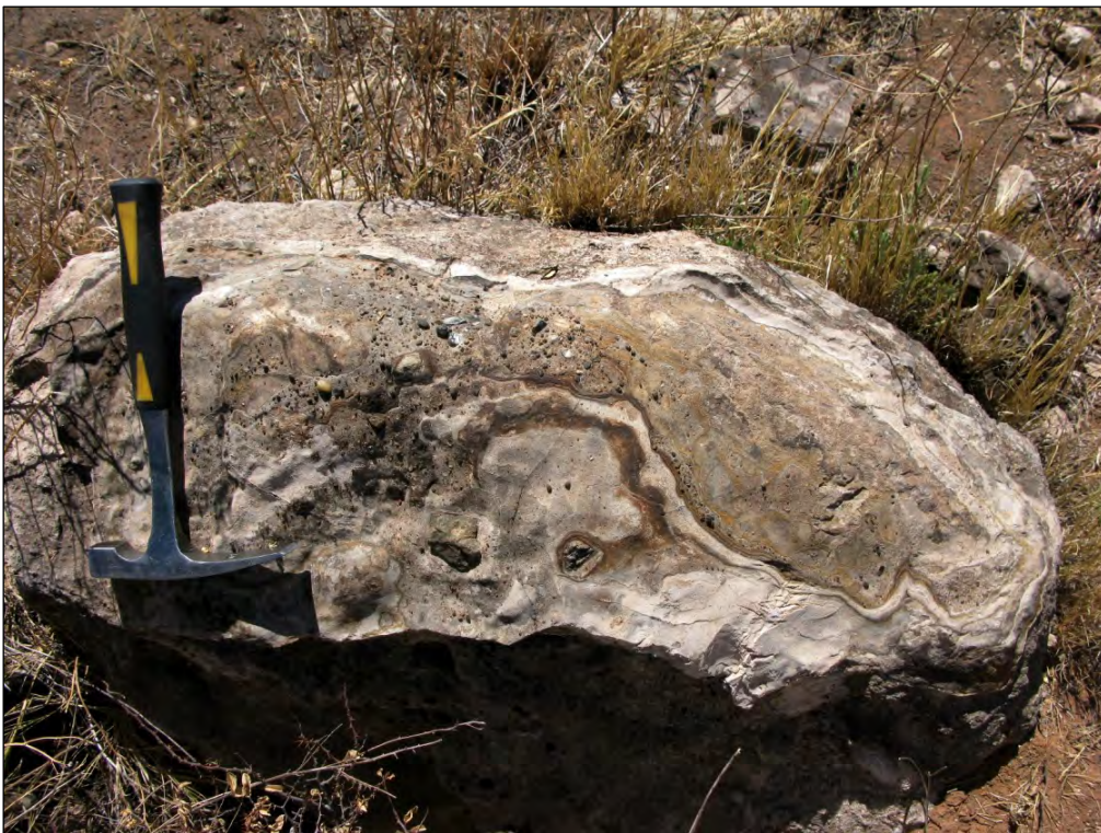
Fig. 59. Displaced block of karstified calcrete hardpan with solution hollows infilled by calcretised gravelly sediment, Trewil Borrow Pit 2 study area (Hammer = c. 30 cm).
