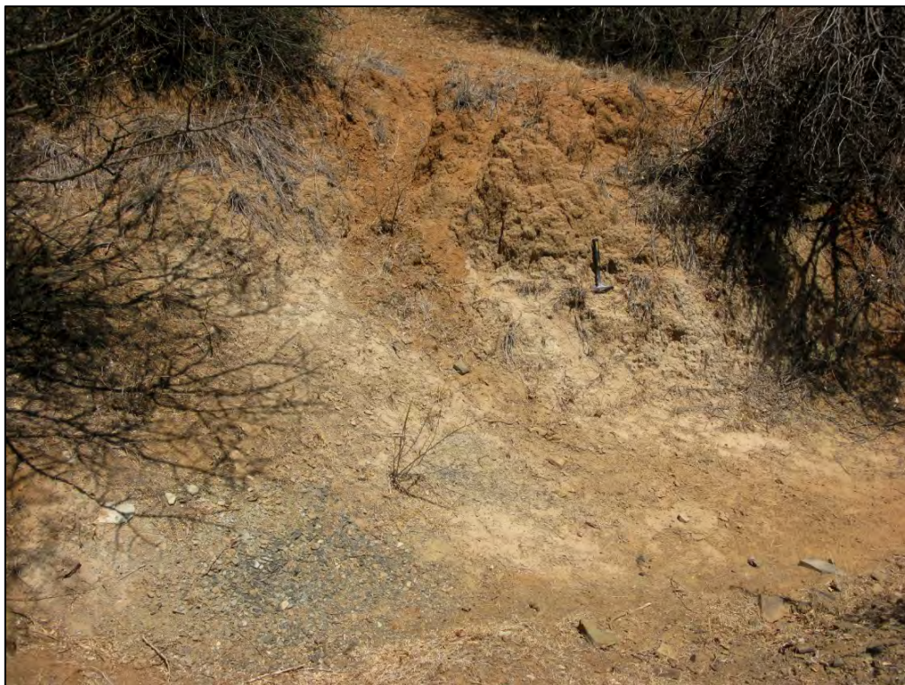
Fig. 53. Pale buff alluvial silts of the Vaal River overlying Karoo mudrocks (bottom RHS) and overlain in turn by orange-brown Hutton sands, western side of Fieldsview borrow pit (Hammer = c. 30 cm).
