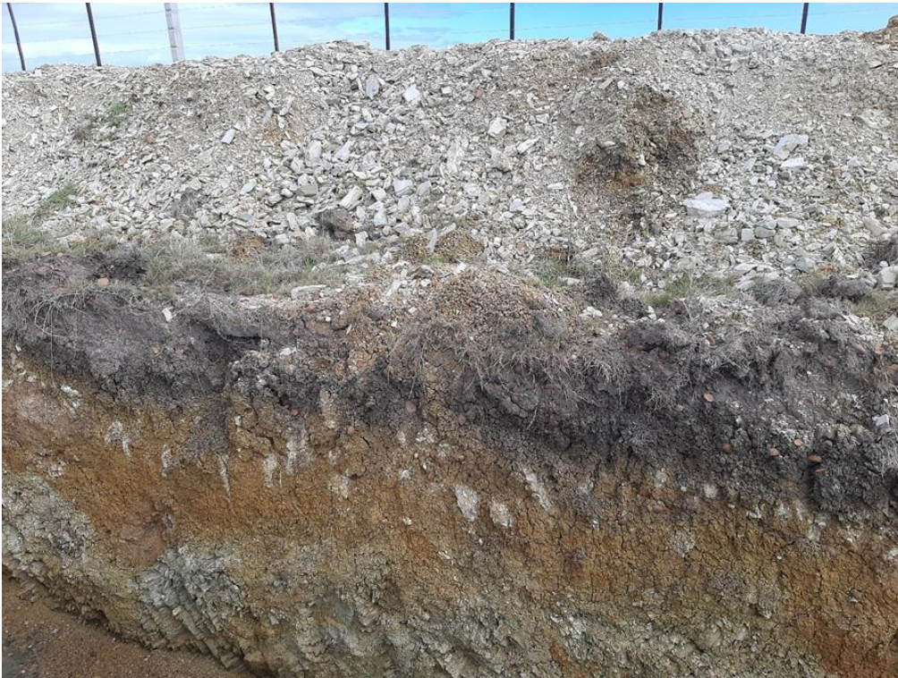
Figure 5: Soil cover and friable rock exposed in ditch next to road at 34°02'53.77"S 24°53'19.23"E
