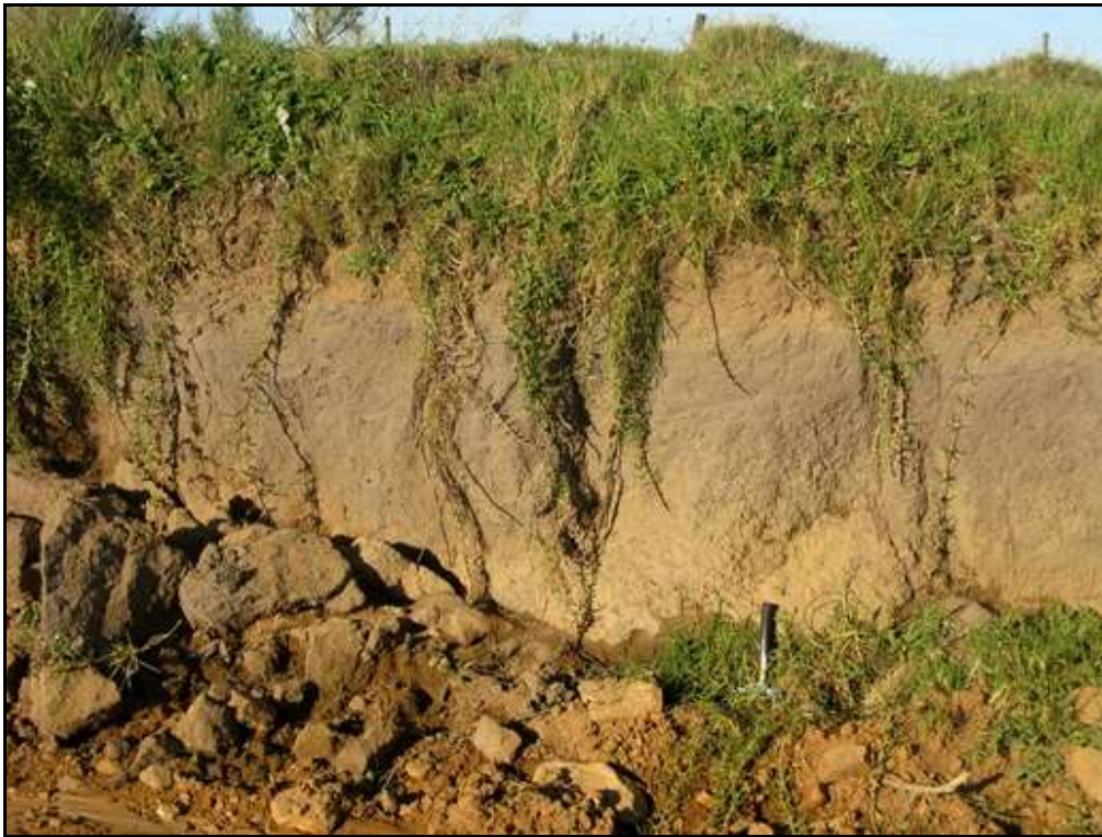
Fig. 19. Thick, brown, silty modern soils with no gravels overlying the Peninsula Formation outcrop area, roadcutting on Zalverige Valley 660/19 (Hammer = 29 cm).
