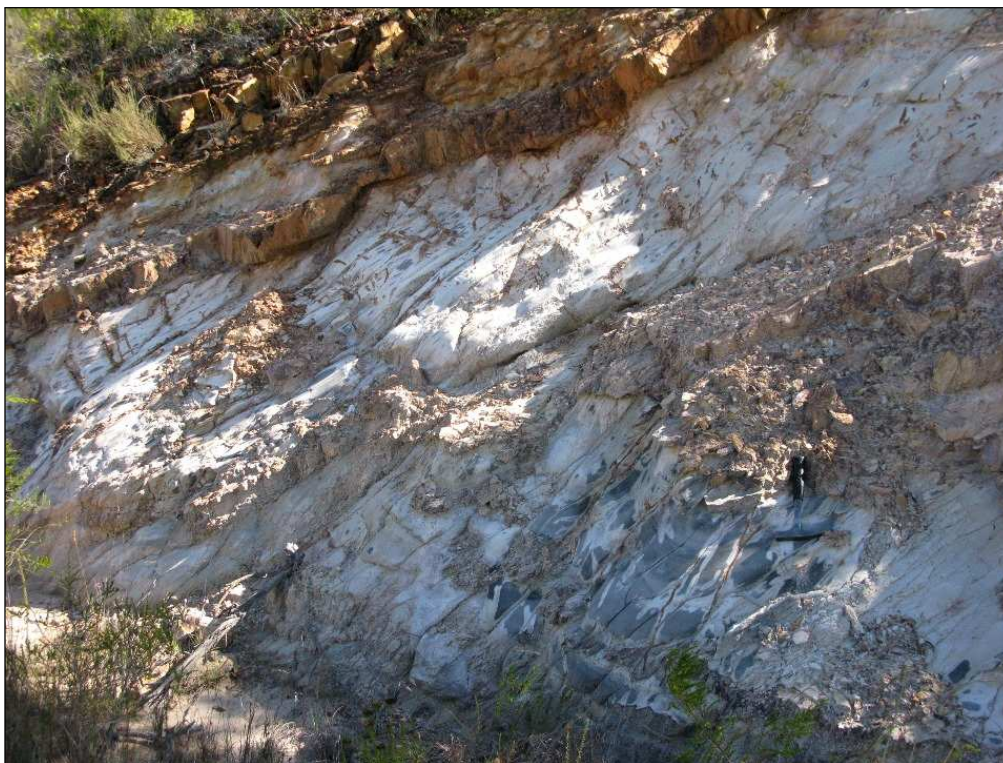
Fig. 4. Deeply-weathered, kaolinitised mudrocks of the Cederberg Formation with thin sandstone interbeds towards the top, R330 road cutting near Weltevrede (Loc. 054) (Hammer = 27 cm).
