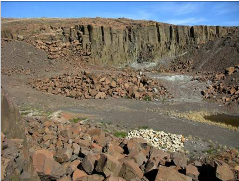
Fig. 12. General view towards the south of the hardrock quarry HRQ1 which is excavated into a major subhorizontal dolerite sill (Loc. 550). Note well developed vertical columnar jointing in the rear quarry face.
