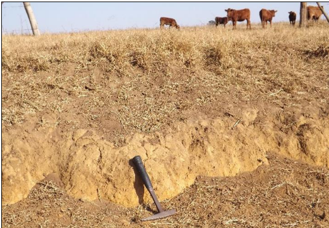
Figure 5: Very weathered dolerite exposed on the right (south) bank highwater slipway.
