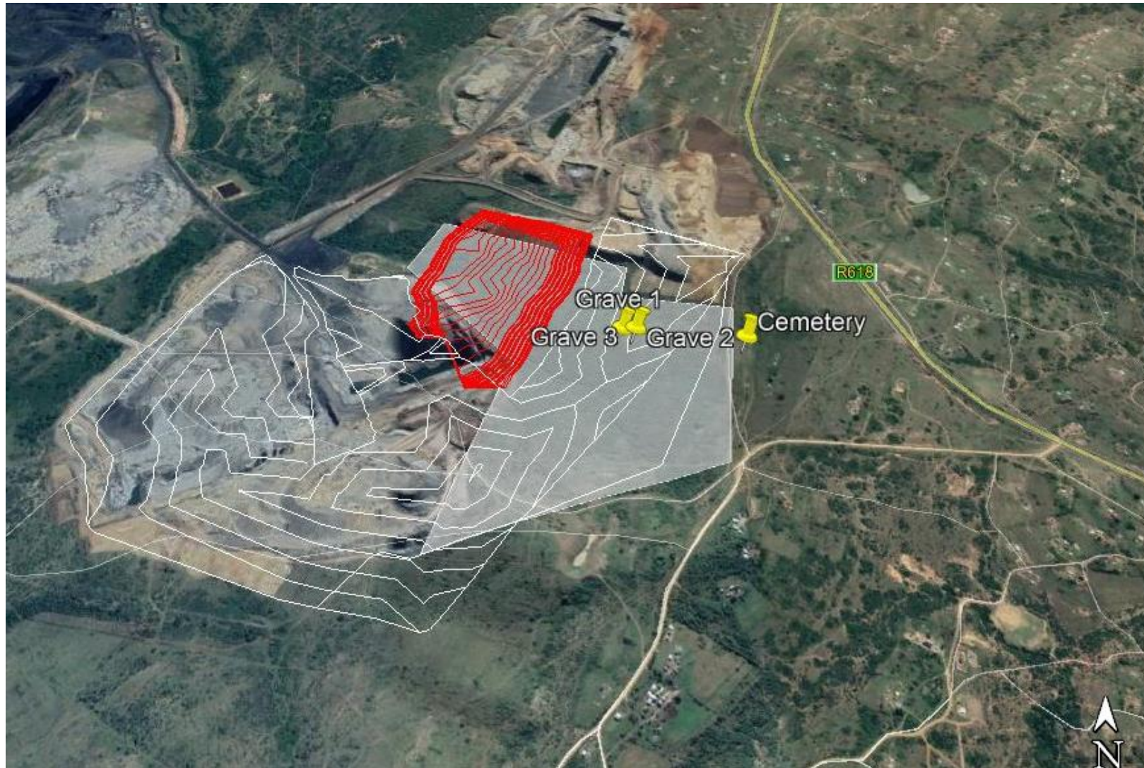
Figure 2: View of Area 8 pit extension shaded in grey with red lines indicating existing pit and white lines the waste rock dump
