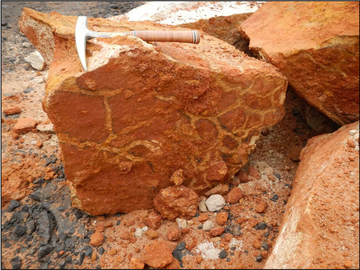
Figure 6.7 Snuff-box weathering in the coarse-grained sandstone of the Vryheid Formation (GPS: S26° 03' 41.5" E28° 53' 07.5")
