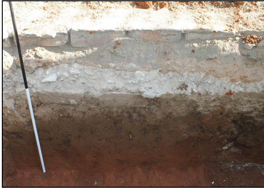
Figure 14: Profile of Test Pit 4 indicating the layer of building rubble under the brick paving and below this another layer of bricks. These lower bricks contain the V incised “frogs”.
