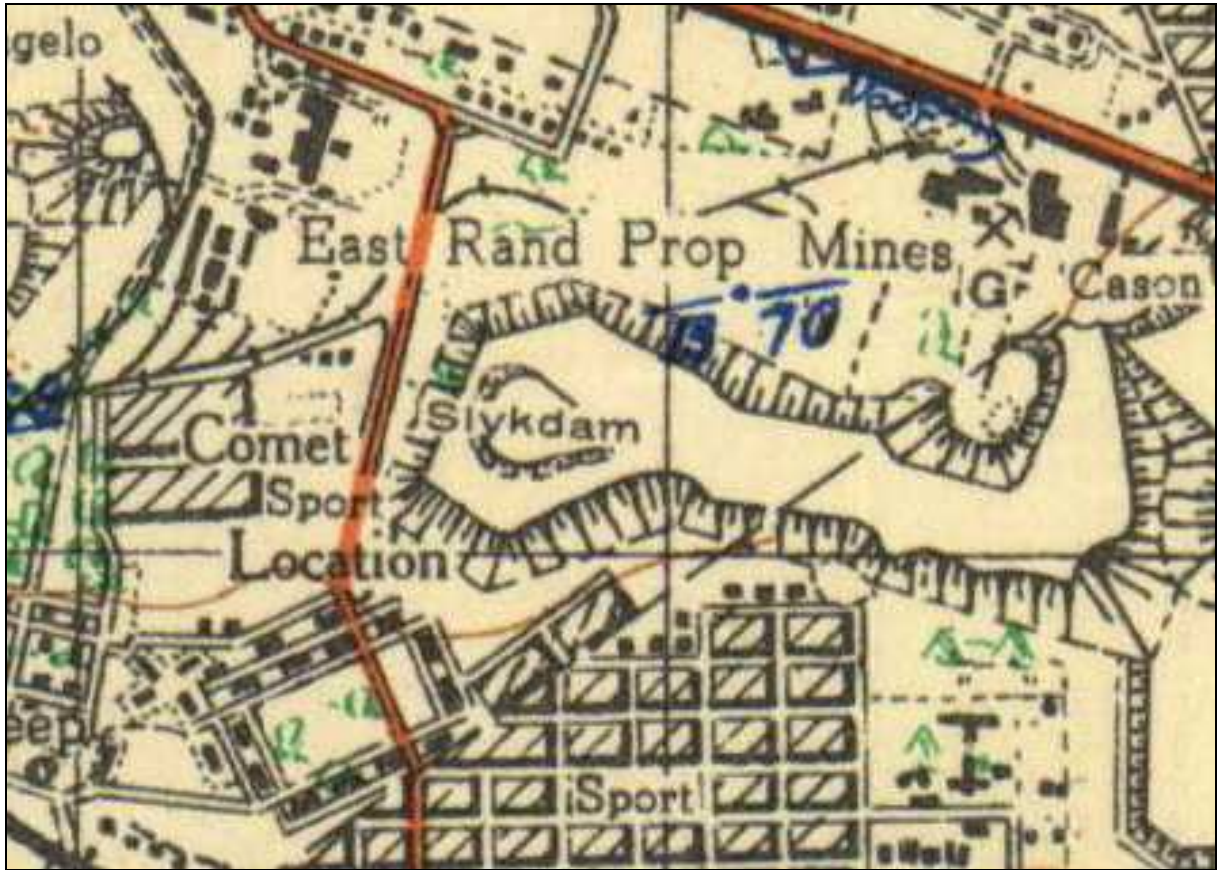
Figure 19 Enlarged section of the Second Edition of the 2628AA Johannesburg sheet of the 1:50 000 topographical map series. This map was surveyed in 1939, and printed in 1945. It represents the earliest available map which depicts the slimes dams within the study area.
