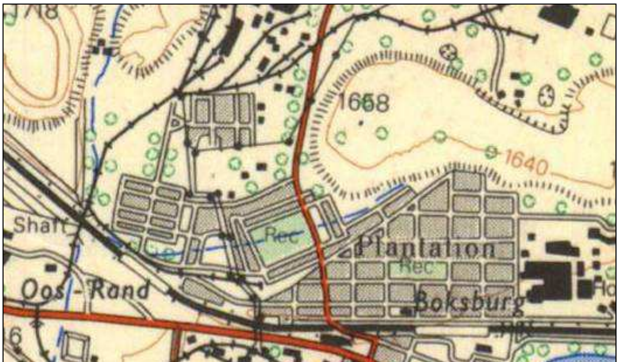
Figure 29 Enlarged section of the Fifth Edition of the 2628AA Topographical Sheet that was compiled during 1975 and printed during 1980. It shows a storm drain, drainage line or watercourse to the south of the slimes dam in exactly the same position as the one depicted on the 1958 map.
