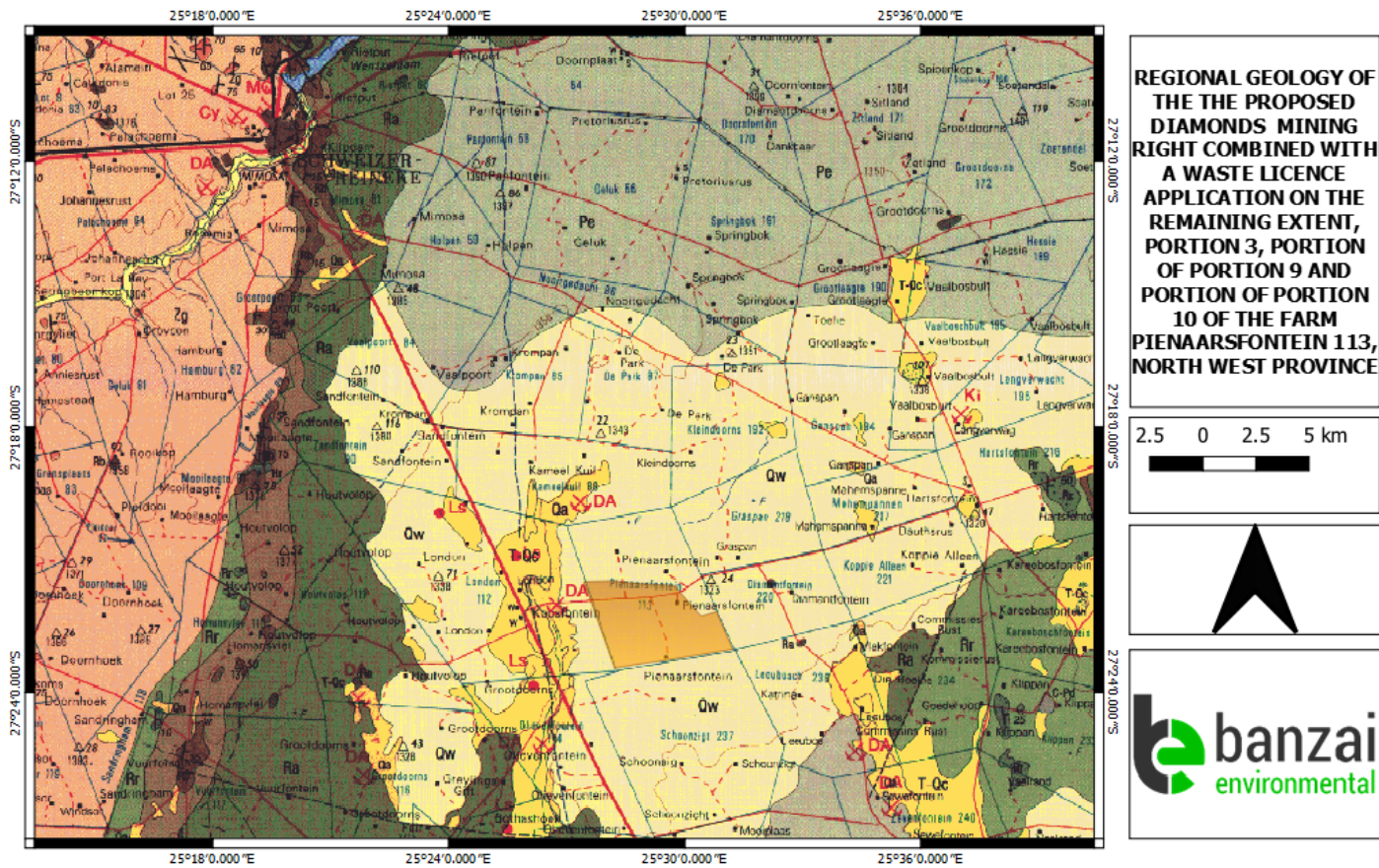
Figure 3: Extract of the 1:250 000 2725 Christiana Geological map (1994) (Council of Geoscience) indicating the proposed development in orange. Surface geology indicates that the development footprint is underlain by the Quaternary aeolian sand (Qw).
