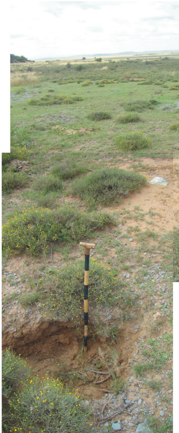
Figure 9. In situ superficial sediments at the site are made up of geologically recent alluvium and residual soils.
