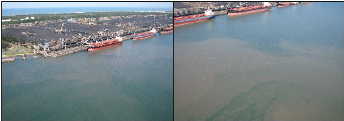
Figure 6.2: Sediment driven into suspension by ship berthing activities in the coal basin in the Port of Richards Bay (photo taken 24th April 2008) (Source: Weerts (2008)).
