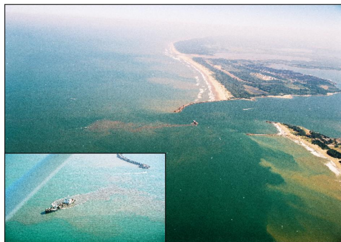
Figure 6.3: Elevated water column turbidity due to dredging activities at the port entrance and re-suspension of sediments in the nearshore environment (Photo courtesy of Mr C.J. Ward as reported in Weerts (2008)).
