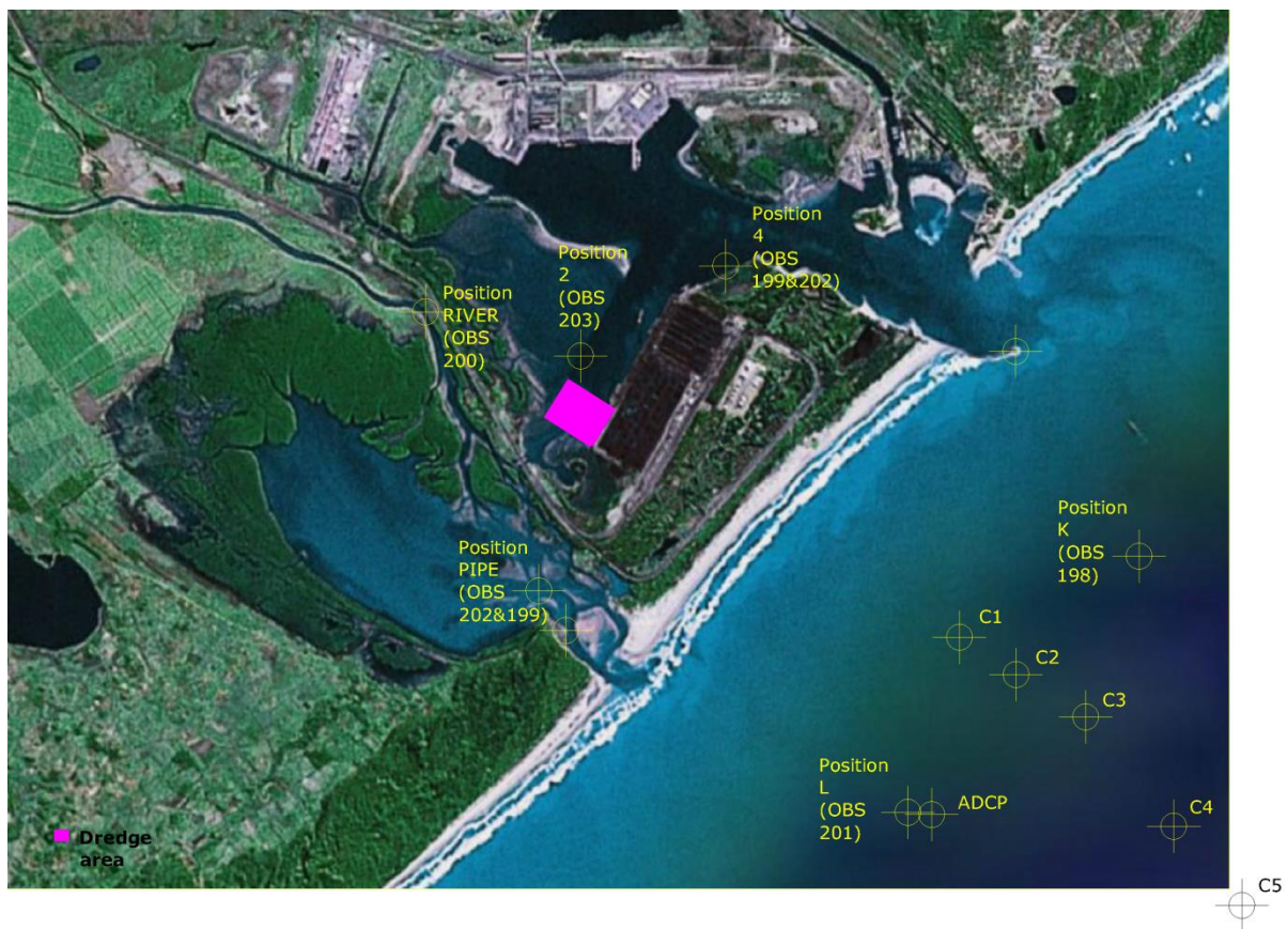
Figure 3.32: Locations of the OBS moorings K and L during the Berth 306 Dredge monitoring programme.
