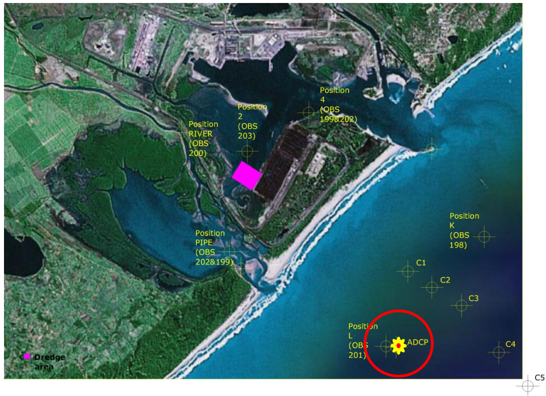
Figure 5.11: Location of the ADCP measurements used both to force and calibrated the hydrodynamic model.
