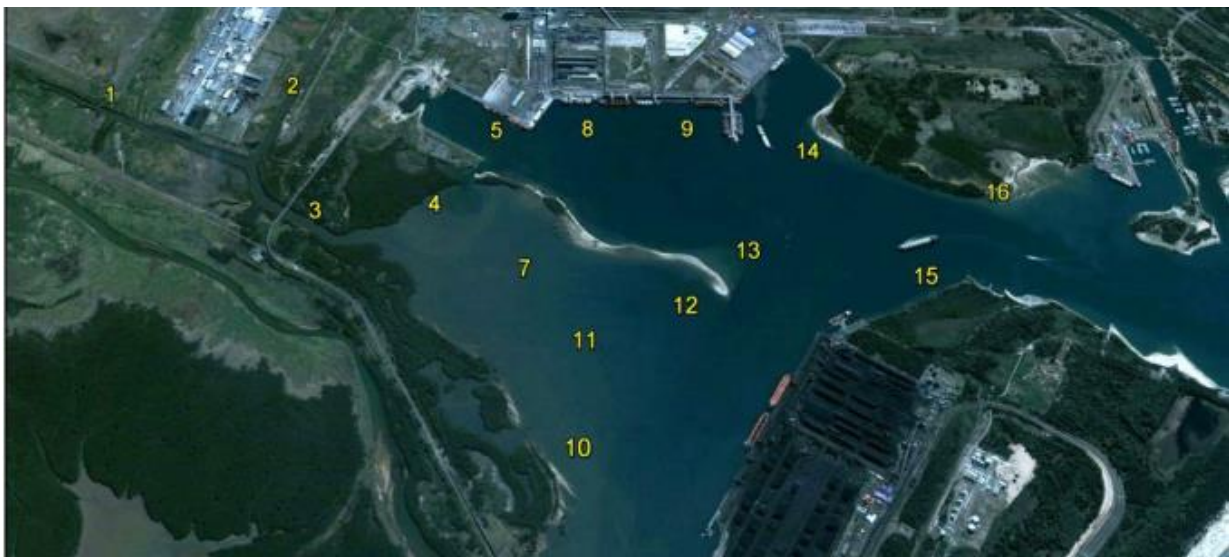
Figure 3.29: Locations in the Port of Richards Bay where turbidity profiling and water sampling for the laboratory measurement of turbidity and analysis of suspended sediment concentrations.
