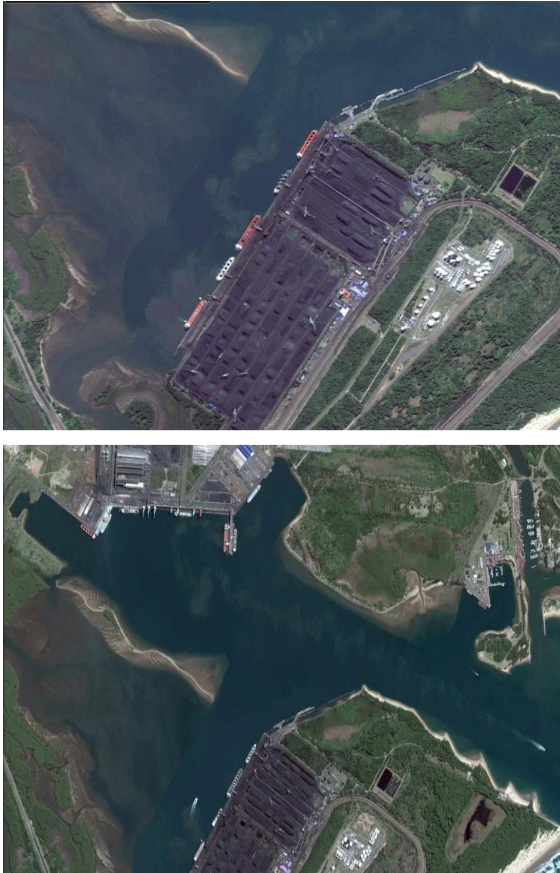
Figure 6.3: Sediment driven into suspension by ship berthing activities in the coal basin (upper panel) in the Port of Richards Bay (GoogleEarth image: 3 May 2014) and in the entrance channel (lower panel) of the Port of Richards Bay (GoogleEarth image: 5 May 2015).
