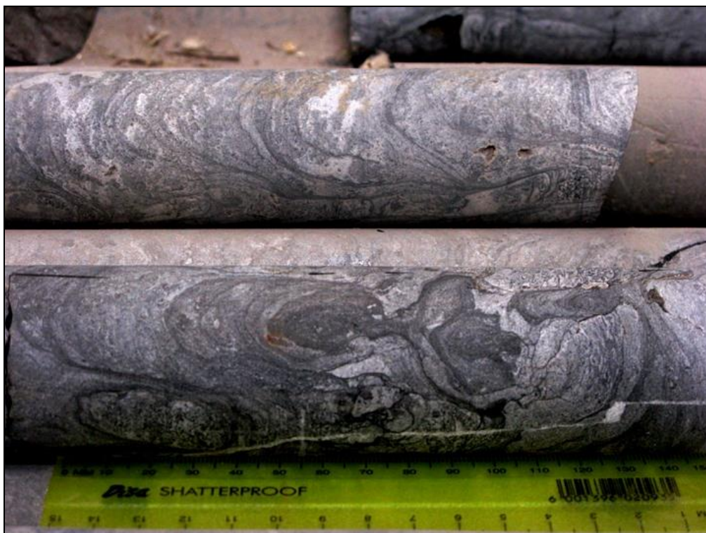
Fig. 33. Borehole cores through a stromatolitic horizon within the Kogelbeen Formation, Lime Acres, showing fine carbonaceous lamination building up towards the left (Scale in cm).
