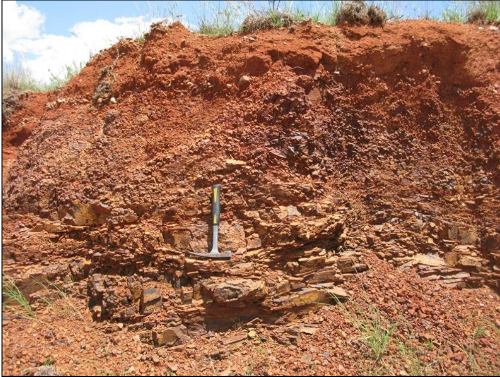
Fig. 23. Deeply-weathered Ongeluk Formation lava saprolite at level of hammer overlain by gravelly soils and orange-brown Kalahari sands (Loc.092) (Hammer = 30 cm).
