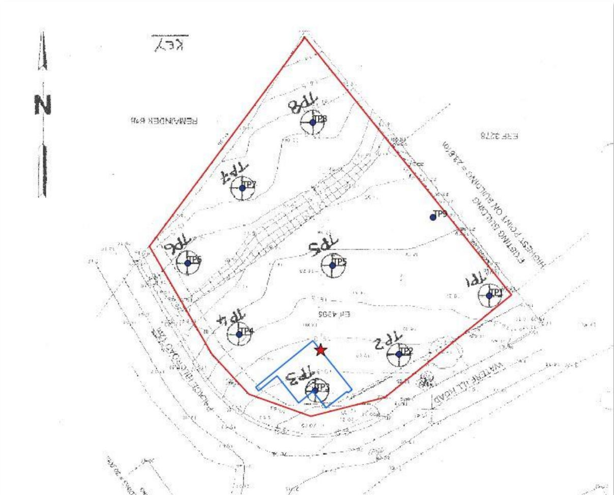
Figure 3: Surveyor General diagram showing the 2006 geotechnical test pit locations, the new foundation trenches and the position of the bone notes by ACO Associates
