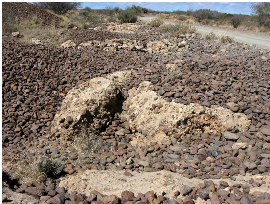
Fig. 17. Previous alluvial diamond mining area on Zwem Kuil 37 showing (reworked) coarse BIF gravels blanketing the potholed calcrete hardpan surface (Loc. 365).
