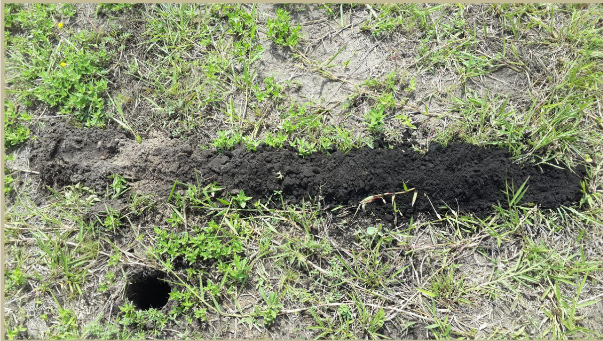
Soil Profile – Aeolian sand overburden grading to a humic sandy clay horizon indicating episodic waterlogged conditions
