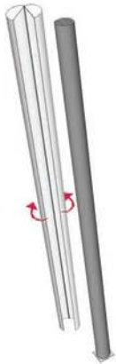
Step 4 mould removed from concrete
