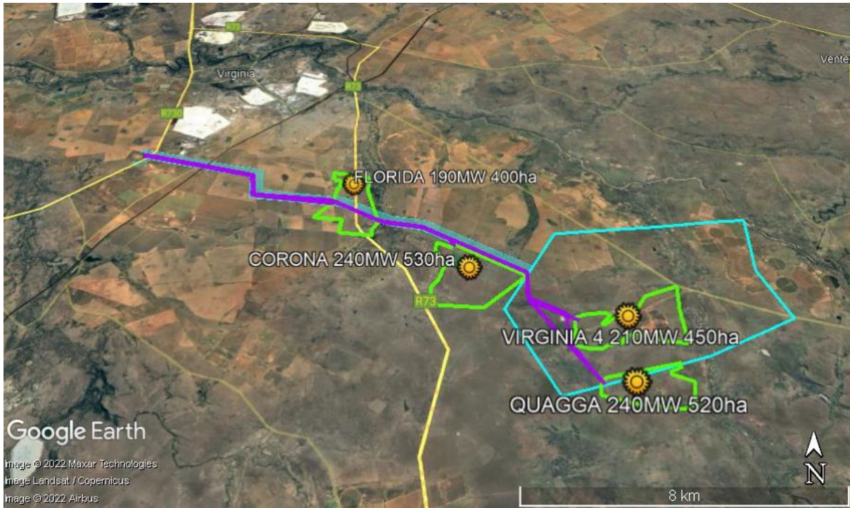
Figure 1: Google Earth map of the proposed Virginia Solar part with the four separate parks (green outlines) with the grid connection (purple lines).
