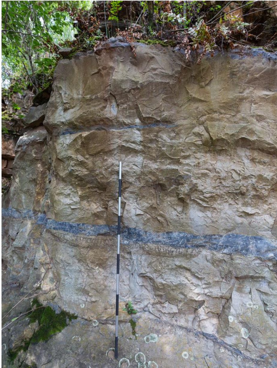
Figure 20. Vertical wall of limestone in an area of the quarry mined pre-1936. Also note the horizontal chert layers. The spall marks are indicative of hand mining by hammer and chisel.
