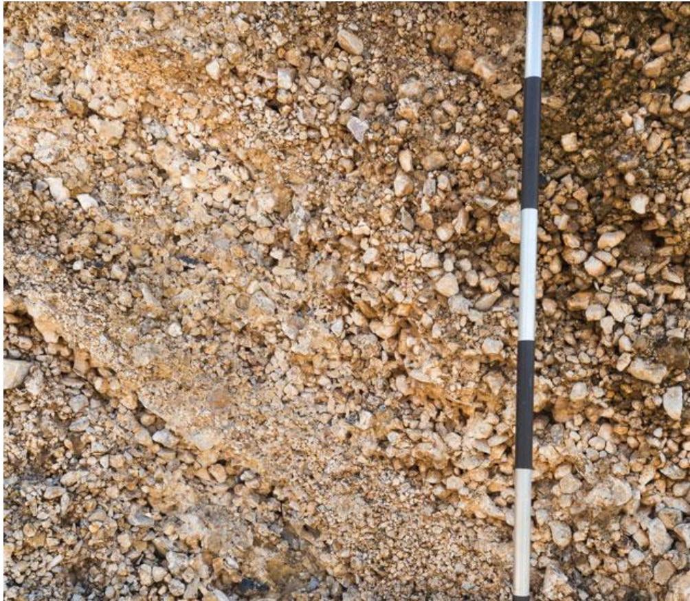
Figure 65. Fine screened material ranging in size from 5 mm to 20 mm.
