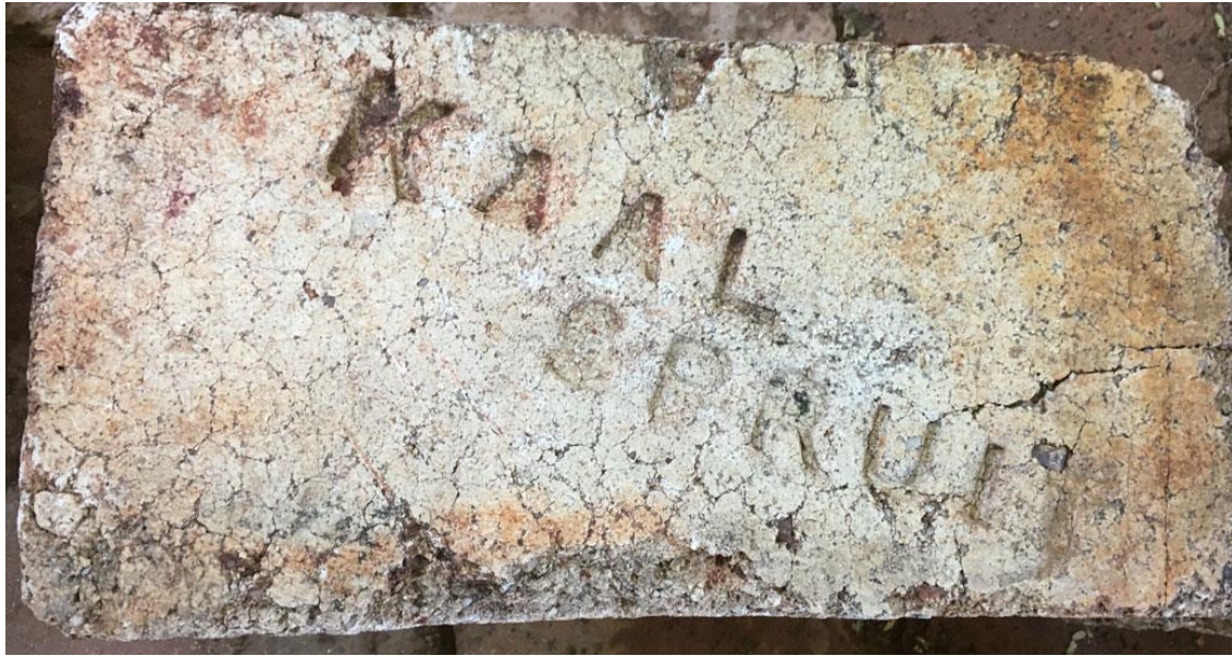
Figure 33. Kaal Spruit brick manufactured between 1896 and 1902. Although extrusion marks are not clear the warping and cracking of the brick allude to the manufacturing process.
