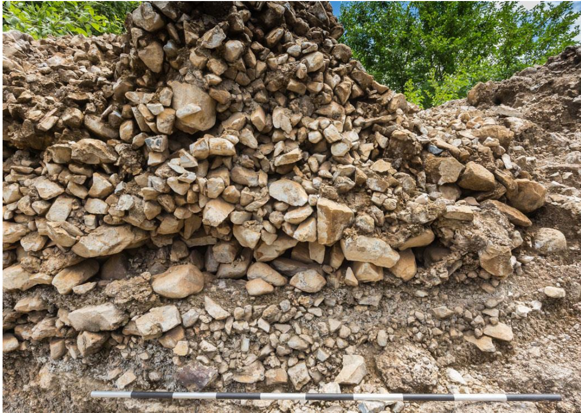
Figure 64. Coarse screened material ranging in size from 150 mm, 75 mm, 50 mm and 20 mm.
