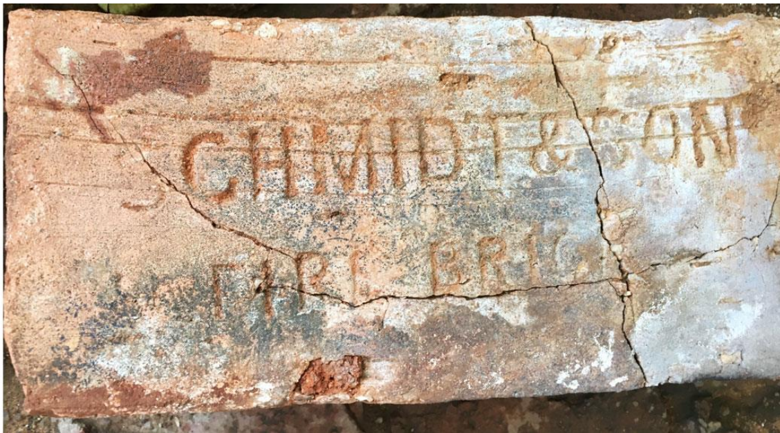
Figure 32. A brick produced by Schmidt & Son Fire Brick Co. that likely dates to the 1890s. Note the horizontal extrusion marks and also warping of the brick.
