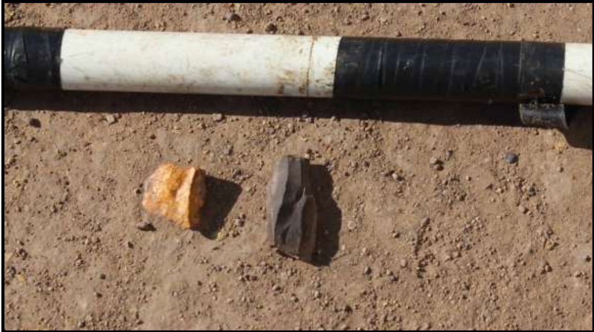
FIG. 23: LSA CORES AT BORROW PIT 2
