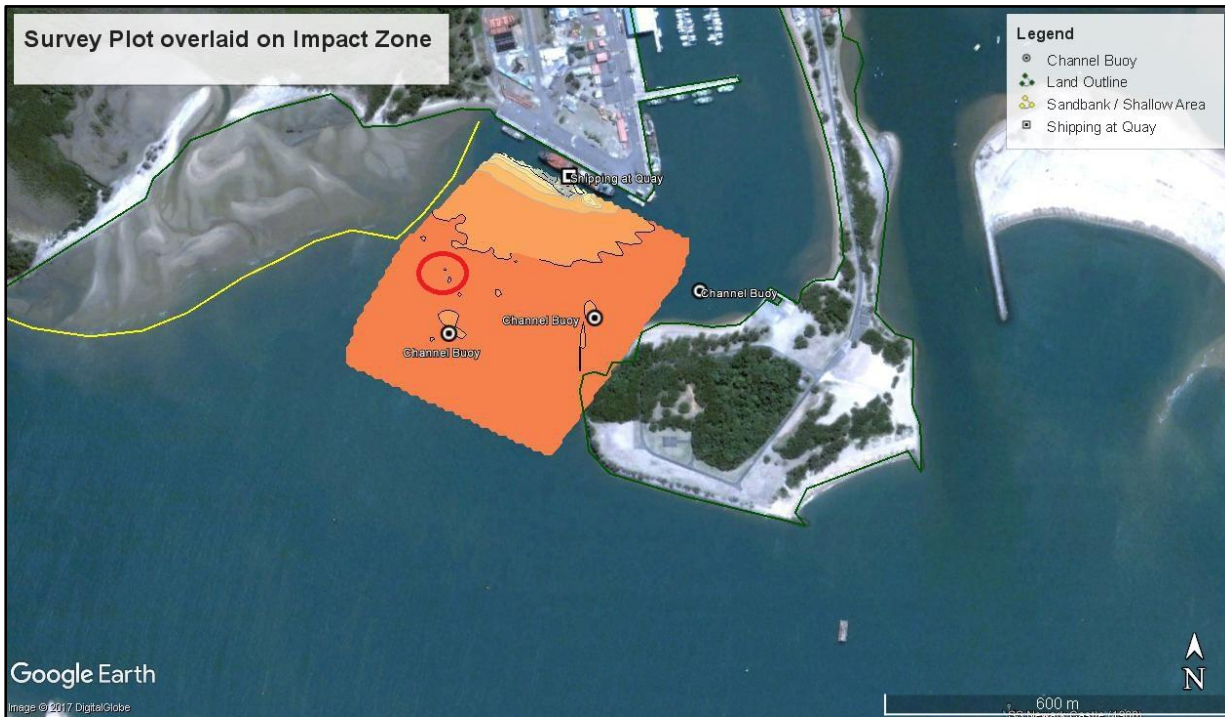
Figure 9: Magnetometer survey with highlighted anomaly (Google Earth: 2017)
