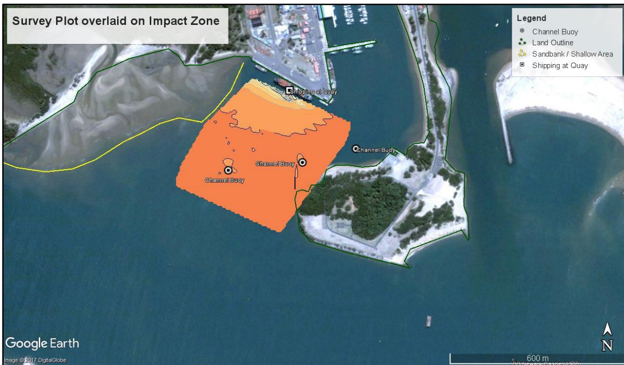
Figure 8: Magnetometer survey with environmental condition plotted (Google Earth: 2017)
