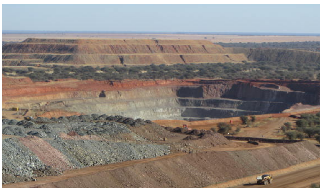
Figure 11. The above image is the A- Zone pit with waste dump facility to its west. This image demonstrates the “opencast” character of this goldmine.
