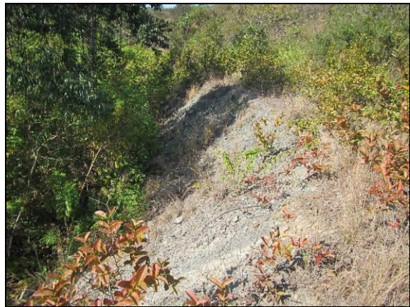
Figure 20: Waste Rock and Tailings material in and adjacent to the drainage line at and downstream of the Old Fairview Plant
