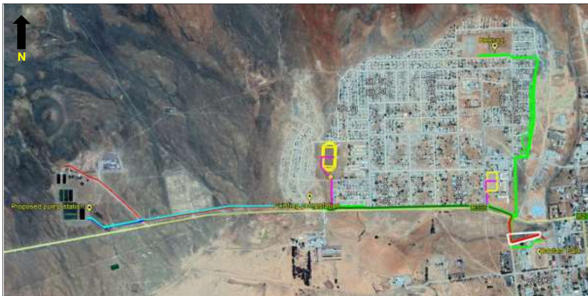
Figure 2. Google satellite map indicating the proposed sewer route (green & purple) for the Calvinia Sports Field Irrigation Project. The light blue line is the existing sewer pipeline from the WWTW. The dark blue line is the proposed new 11kV line that will connect to the existing 11kV overhead line (red)
