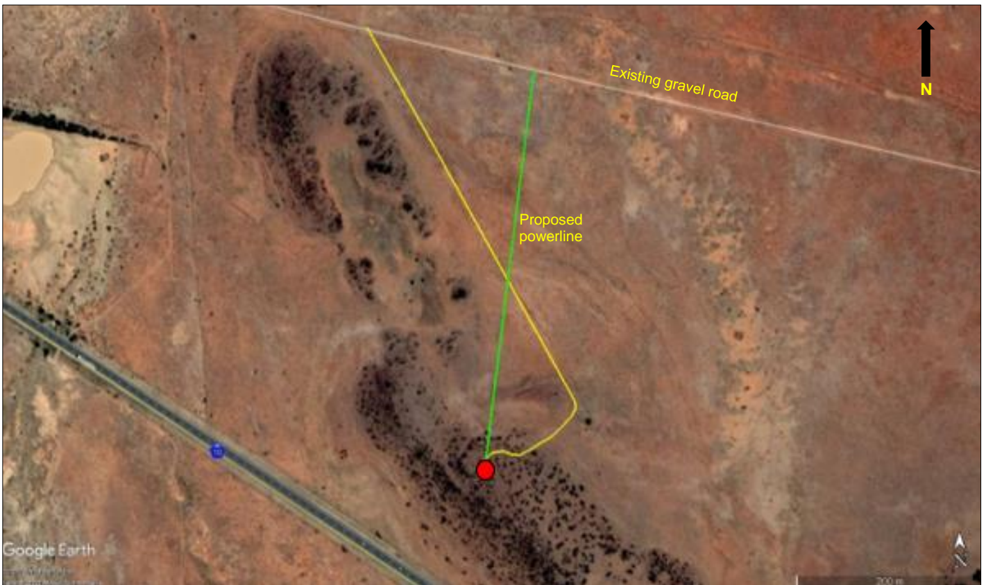
Figure 3. Google Earth image showing the location of the proposed telecommunication mast (red placemark). The proposed 3m wide gravel access road is indicated by the yellow line, and the proposed 420m overhead powerline is indicated by the green line.
