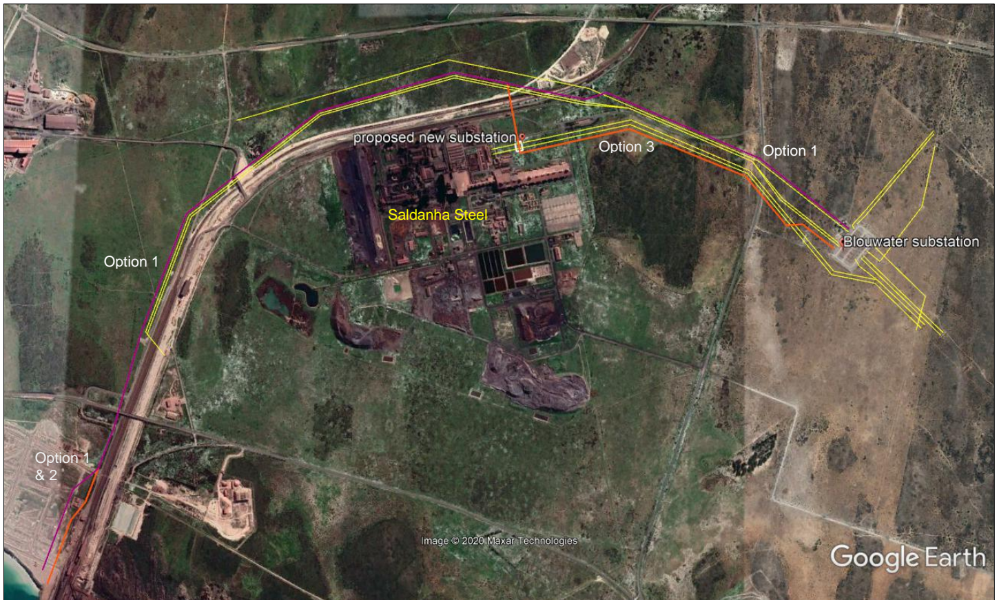
Figure 3. Google satellite map indicating the proposed 132 kV double circuit powerline, Option 1 (Purple), Option 2 (red) & Option 3 (orange). The proposed substation on the Arcelor/Mittal Steel Plant is also indicated. Yellow lines are the existing 66kV and 132 kV overhead powerlines.
