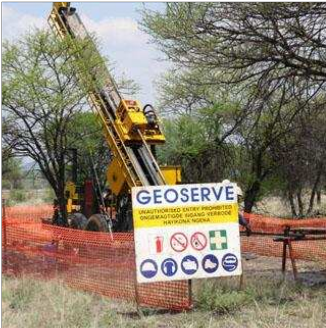
Figure 4. Example of the drill and drilling method to be used on Farm 349
