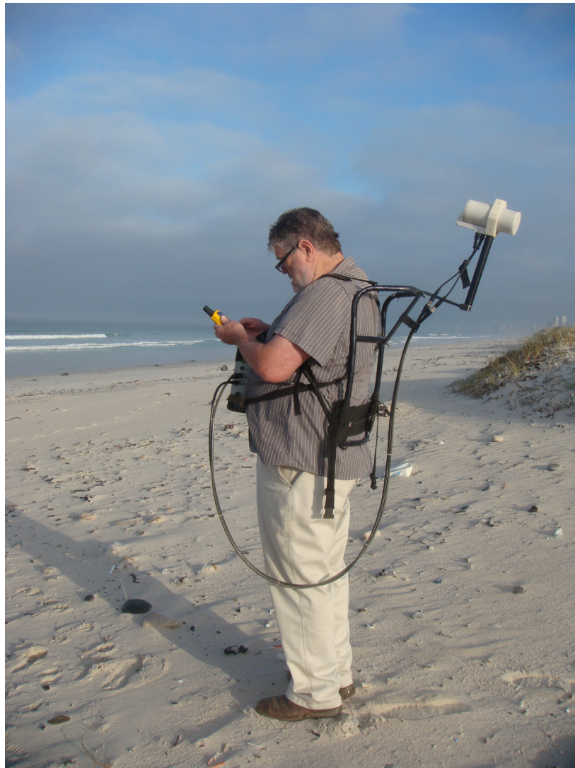
Figure 2: The author with a GEM 19 magnetometer and hand held GPS
