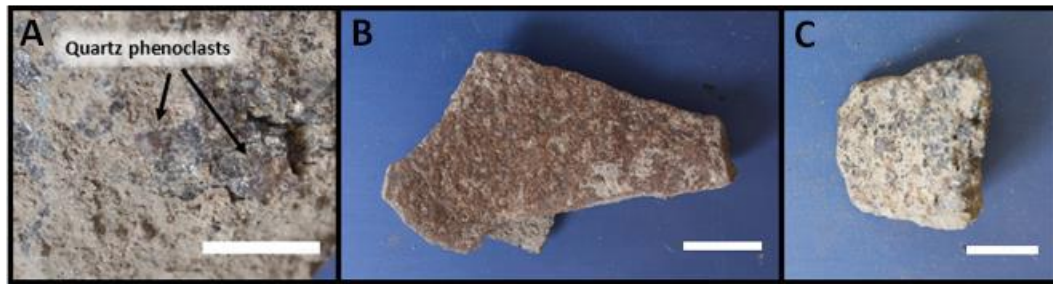
Figure 3: A) No. 2402 showing a coarse-grained texture and quartz phenoclasts. B) No. 1286 and C) No. 2366 are examples of the general characteristics of OBP sandstone lithics. The white bar represents 1 cm.
