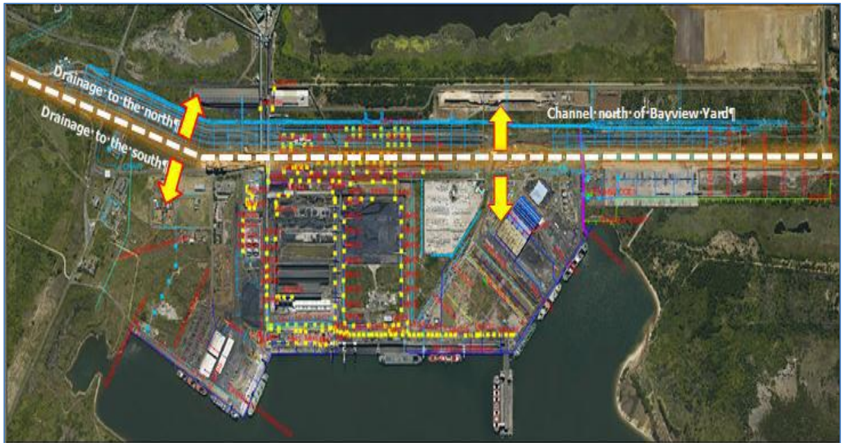
Figure 6-14: Storm water as-built and flow directions
