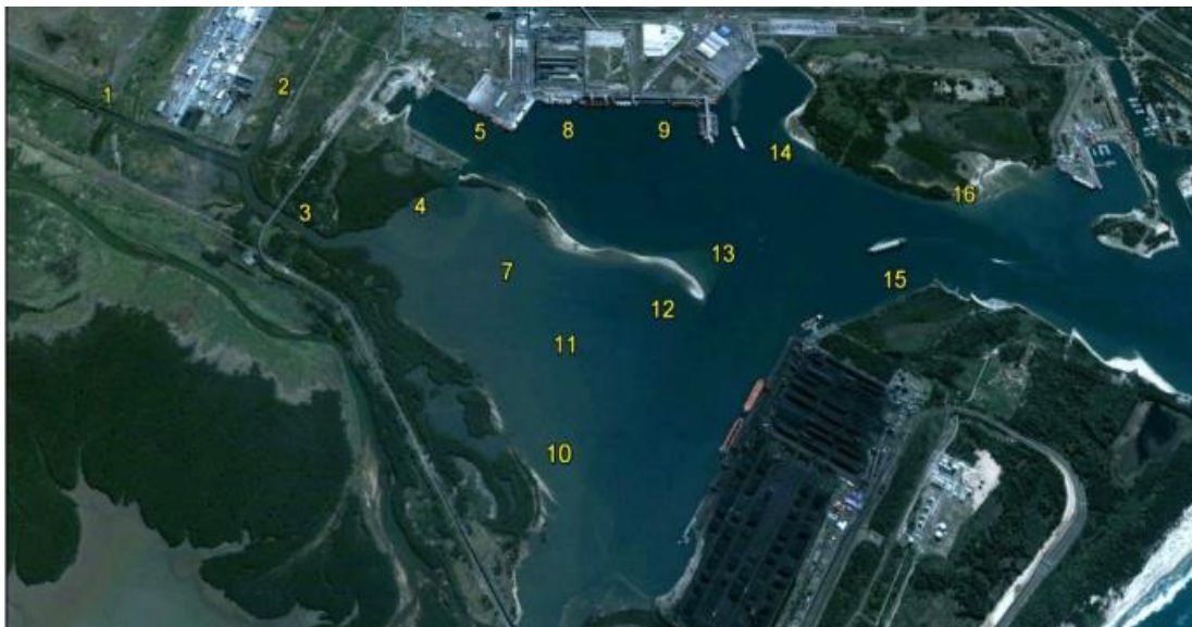
Figure 7-27: Locations in the Port of Richards Bay were turbidity profiling and water sampling for the laboratory measurement of turbidity and analysis of suspended sediment concentrations
