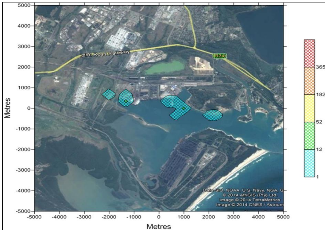
Figure 7-7: Modelled Representation of Incidences of Ambient SO 2 Levels (1 hour average) from Proposed Increased in Shipping Exceeding 87.5 µg/m 3 Level (25% of ambient standard)
