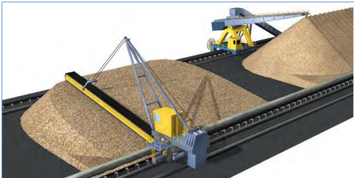
Figure 3-9: Stacker and Scraper Reclaimer System
