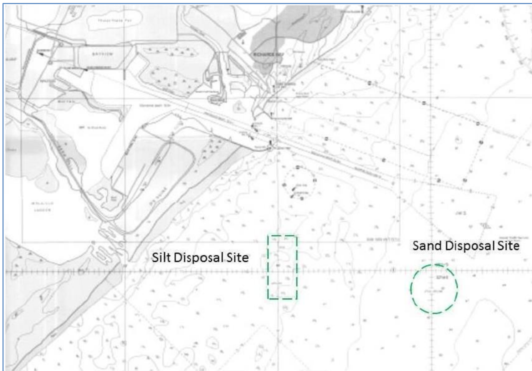
Figure 3-17: Existing Off-Shore Dredge Disposal Site Locations
