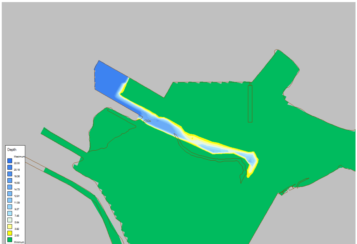
Figure 7-14: Estimated depth of sediment that needs to be dredged or excavated for the Option 3A wide basin layout
