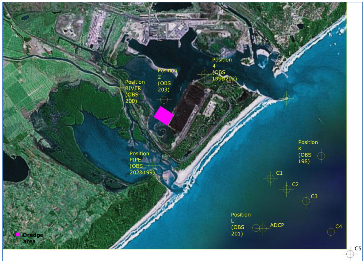
Figure 7-29: Locations of the OBS moorings K and L during the Berth 306 Dredge monitoring programme
