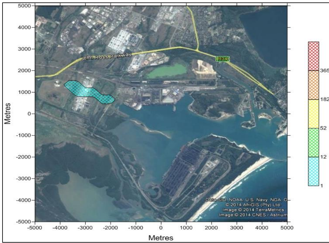
Figure 7-6: Modelled Representation of Incidences of Ambient SO 2 Levels (24 hour average) from the proposed Increased in Shipping Exceeding 31.75 \mu\text{g}/\text{m}^3 Level (25% of ambient standard)
