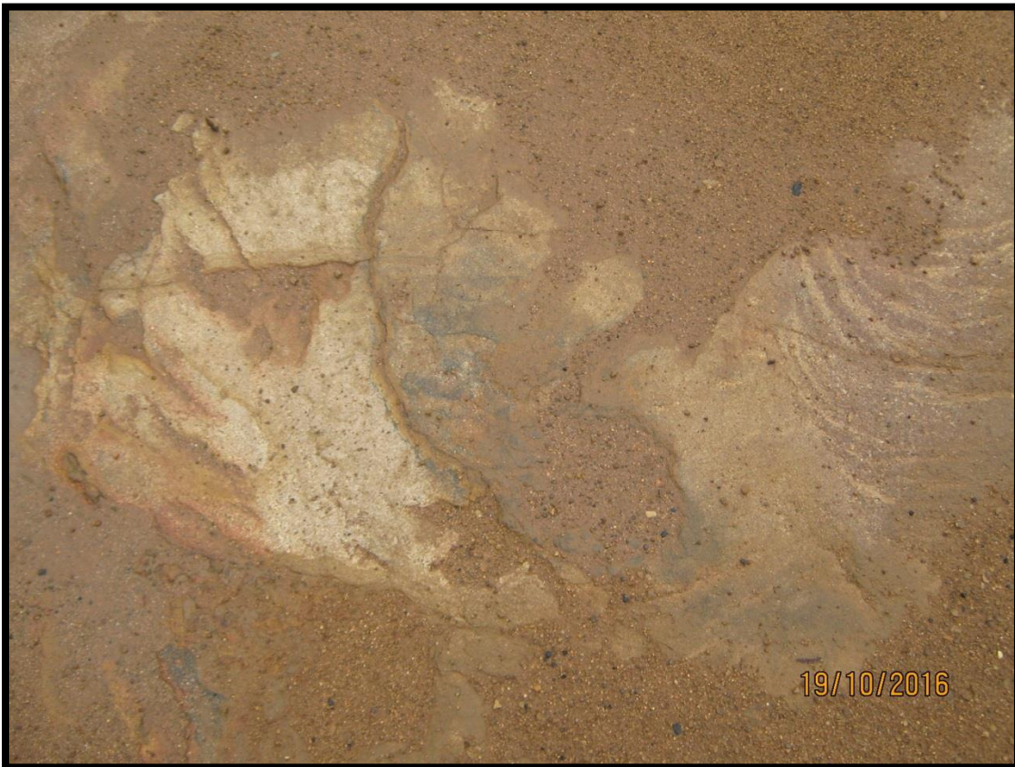
Figure 9: Gritty sandstone on road close to where second road from the R555 Road enters the site at cemetery.
