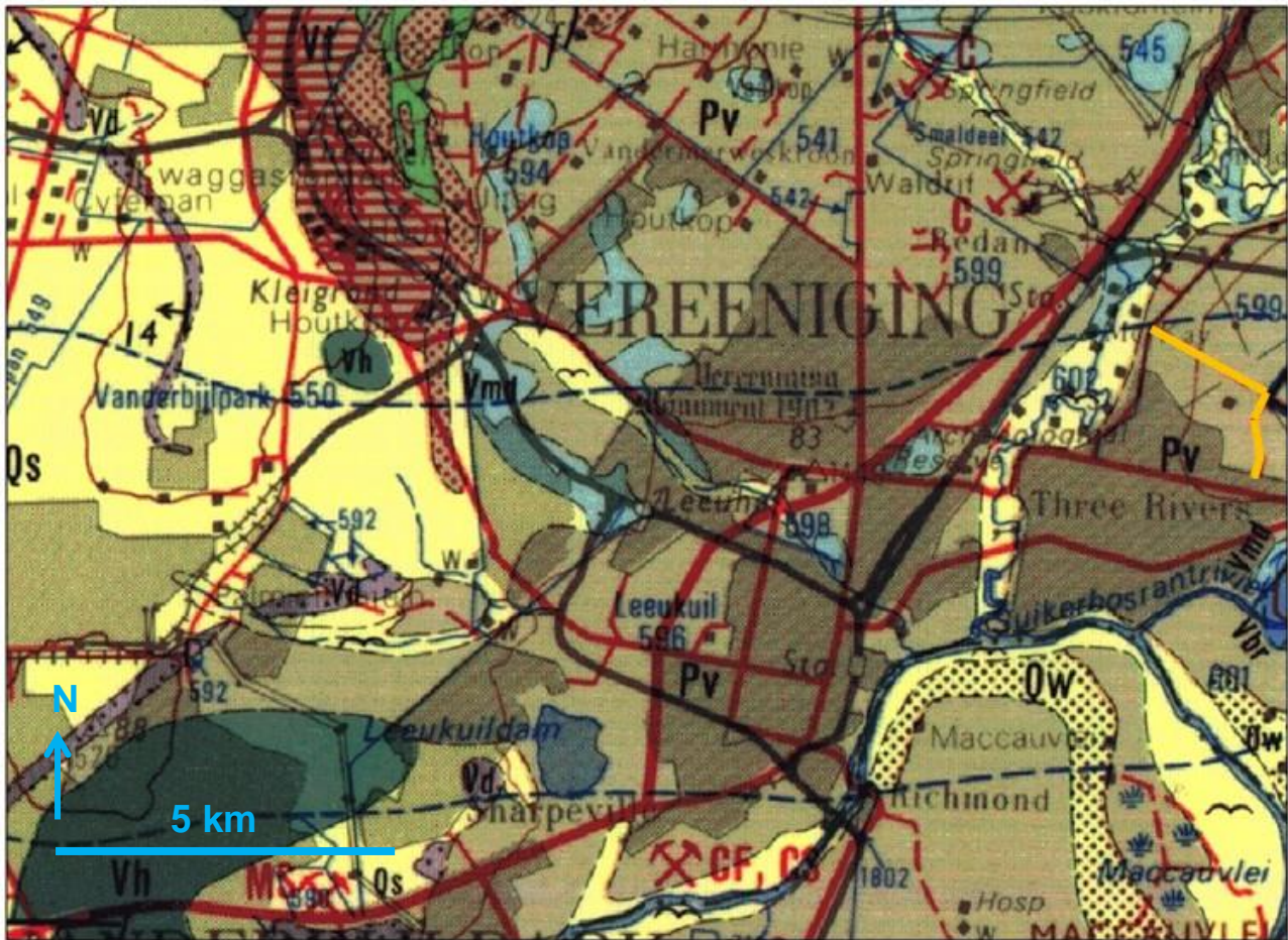
Figure 2: Extract from 1: 250 000 geology sheet 2626 West Rand showing the route of the existing Risiville / McKay 11kV feeder line (orange line) on the NE outskirts of Vereeniging, Gauteng Province. The region is underlain by Middle Permian deltaic sediments of the Vryheid Formation (Ecca Group, Karoo Supergroup) (Pv, grey). A narrow strip of Late Caenozoic alluvium (pale yellow) is associated with a stream tributary of the Suikerbosrantrivier drainage system just to the west.
