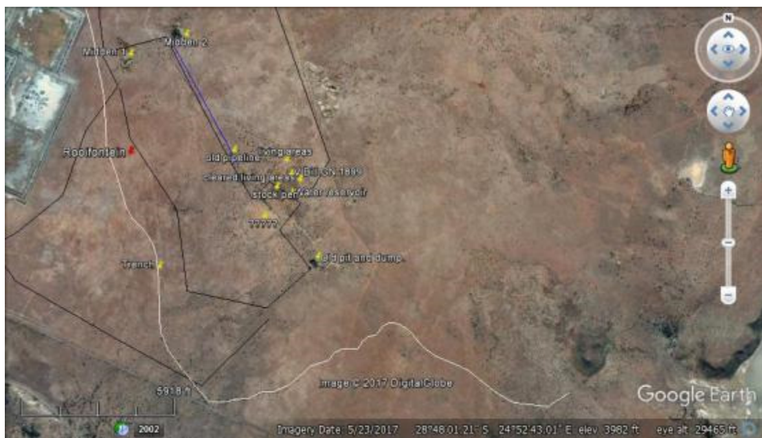
Fig. 63. White line marks a trench that appears to have carried water from a reservoir to the east of Rooifontein to Wesselon mine over a distance of about 10 kilometres. It varies in depth but are constructed on an incline of about 1 : 1000 (Google Earth 2017.)
