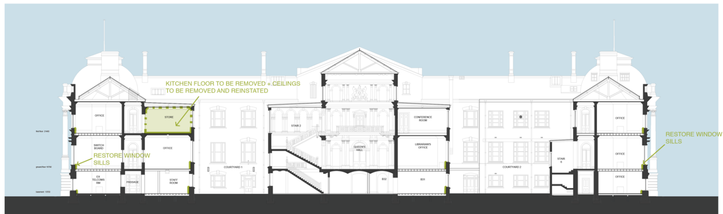
DD: LONGITUDINAL SECTION THROUGH COURTYARDS 1:100
