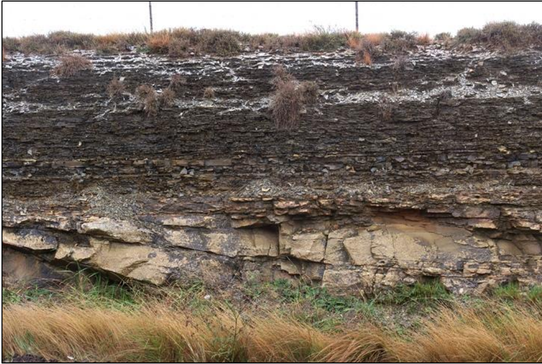
Figure 32: Extension of road cutting illustrated above with a thin, dark grey mudrock interval between the lower, cross-bedded channel sandstone and darker, thinly bedded, tabular facies above.
