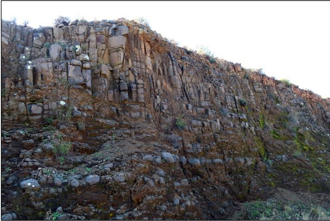
Figure 54: Cut face through a weathered dolerite sill showing intensive jointing and corestone formation, small quarry on Farm 37/63 (WEF 1) near Molteno.
