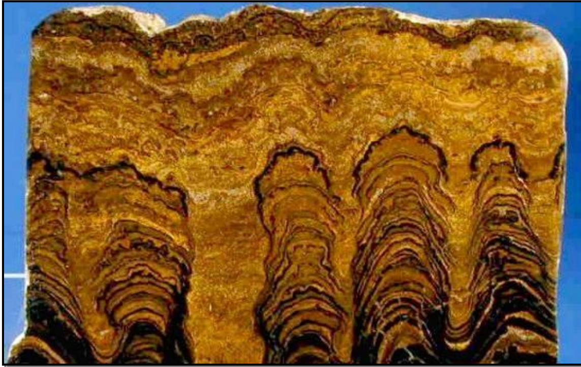
Figure 4.1 Typical stromatolite structures usually associated with dolomite deposits such as the dolomite of the Mooidraai Formation that overlies the Hotazel Formation. It is highly likely that structures such as in this photograph, might be exposed during exposure of the dolomite and Banded Iron Units in the Hotazel Formation (Photograph from Wikipedia 201) en.wikipedia.org/wiki/Stromatolite .
