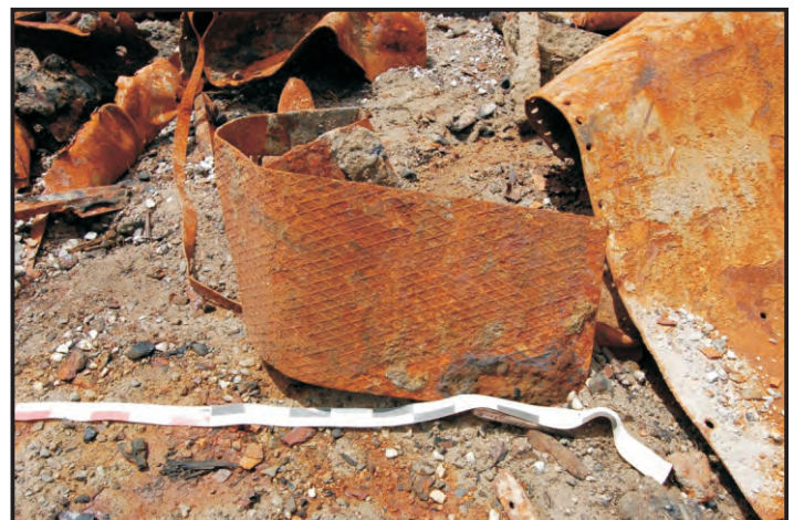
Figure 91: Non-slip sheeting, this would be attached on gangways etc. (Photo: Maitland)
