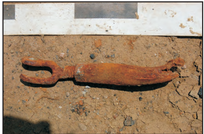
Figures 130 - 131: The opposing ends of a turnbuckle, the first is a fixed eye on the end of a screw and the second is a shackle on the end of a screw. These were used to adjust the tension or length of rigging wires (Manual of Seamanship 1951; Photo: Maitland)
