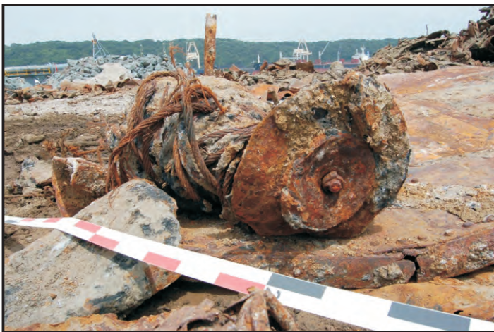
Figures 99 - 100: Steam windlass. According to the Lloyd's Survey of 1921, the Karin had a steam windlass. This was usually placed on the upper fore-castle deck and was used for hauling up bower anchors (Appendix A: 3; Paasch 1890: 156; Photos: Maitland)
