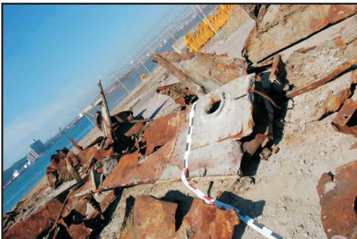
Figures 51 - 52: Top and side view of the bow hawsehole, there is an extra reinforcing plate around it (Photos: Maitland)
