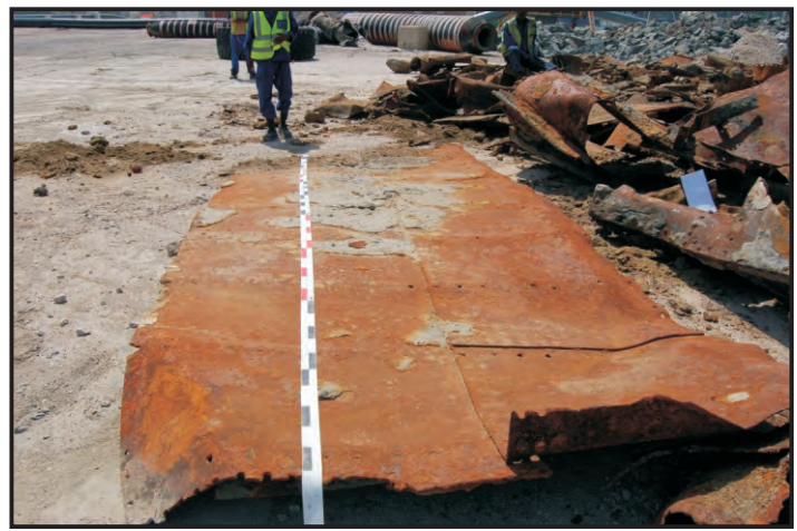
Figure 36: Long section of hull plating, the Karin hull was severely distorted due to post-depositional damage (Photo: Maitland)
