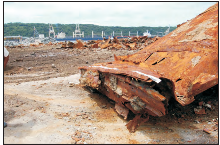
Figure 68: Close-up showing part of the centre keelson (Photo: Maitland)
