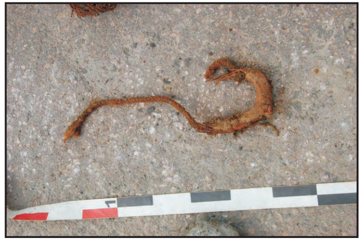
Figure 135: Remains of wire cable with a hemp core that was spliced to form a hawser eye (Manual of Seamanship 1951: 95 - 96; Photo: Maitland)
