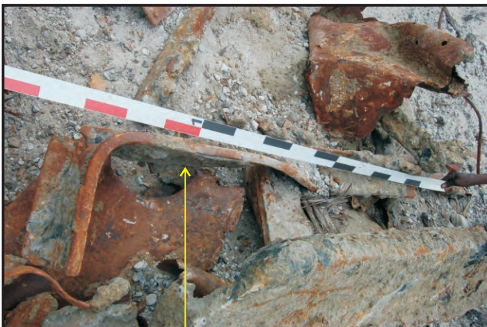
Figure 107: Frame from a watertight door (Manual of Seamanship 1951:47; Photo: Maitland)
