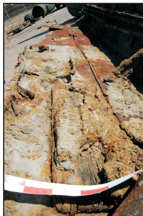
Figure 61: Section of deck plating near the bulwark with wood planks, the wood may have served as a base for deck equipment (Photo: Maitland)
