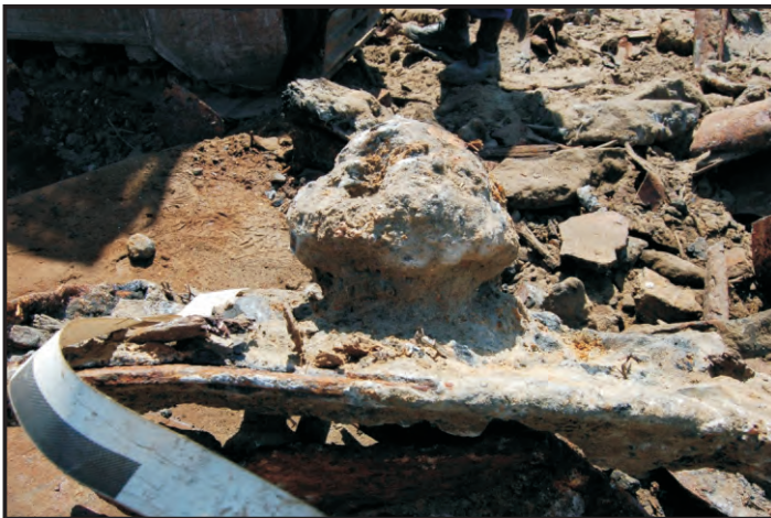
Figure 94 -95: Two deck capstan rollers, the first is still attached to the deck plating (Renda 2010; Photo: Maitland)
