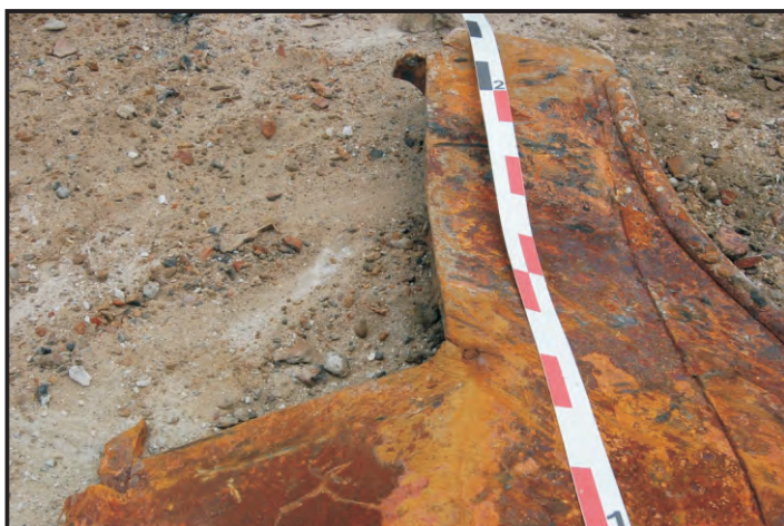
Figure 64: External view of a washport, the curve of the well deck bulwark is also visible (Photo: Maitland)
