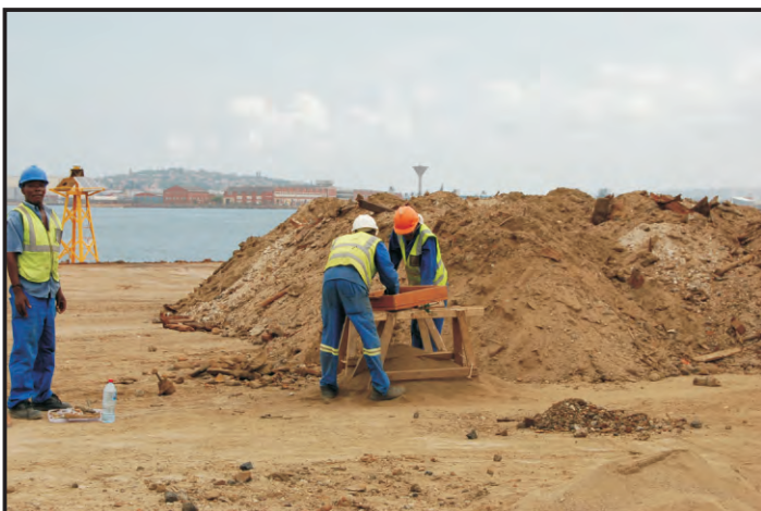
Figure 23: A sample of approximately 1 ton was sifted through a 3mm mesh sieve. However, the cost/benefit of this exercise made it unviable (Photo: Maitland)
