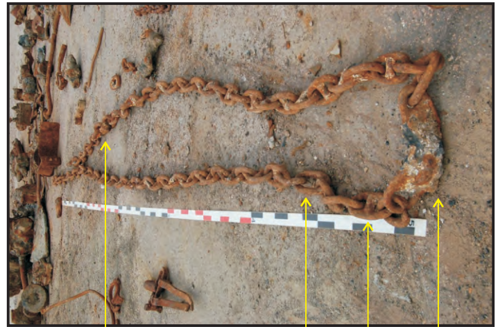
Figure 137: About 10 meters of stud link anchor cable (Paasch 1890: Plate 65; Photo: Maitland)
