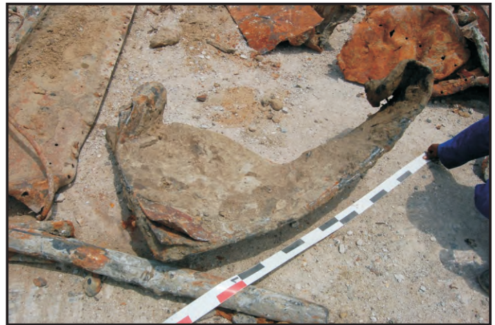
Figure 74: Breasthook or crutch depending on whether it is from the bow or the stern; a plate that strengthens these areas (Photo: Maitland)
