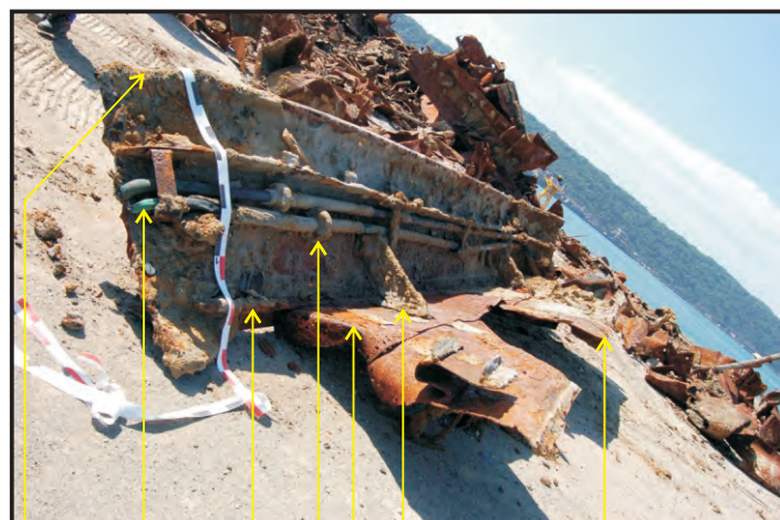
Main rail Bulwark piping Deck stringer plate Coupling flange Gunwale angle bar Bulwark stay Deck plating
