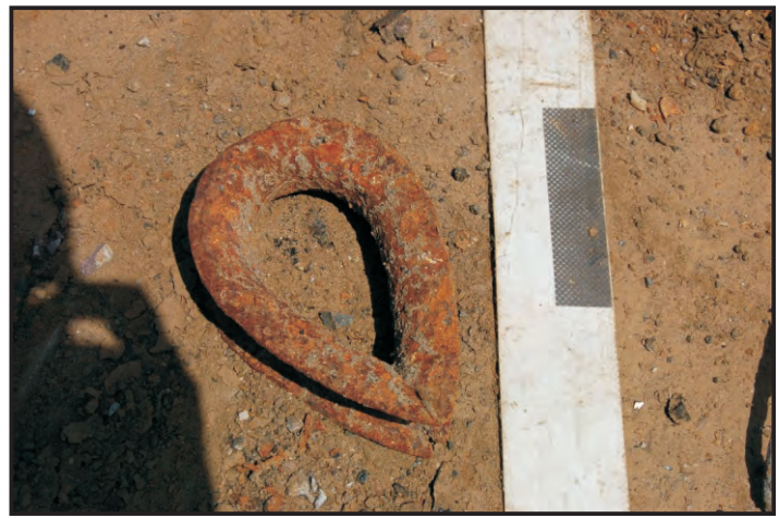
Figure 123: Heart-shaped open thimble (Manual of Seamanship 1951: 169; Photo: Maitland)
