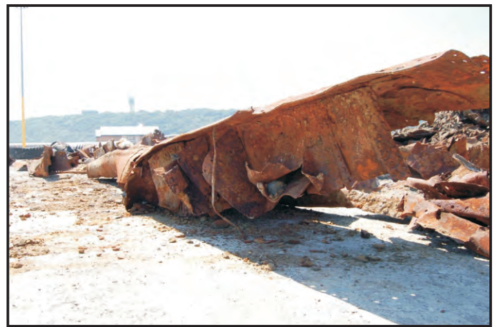
Figure 44: Hull plating with large support structures, possibly from the engine room (Photo: Maitland)
