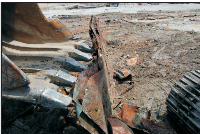
Figure 39: Triple steel plates, thinner than the hull plating (Photo: Maitland)
