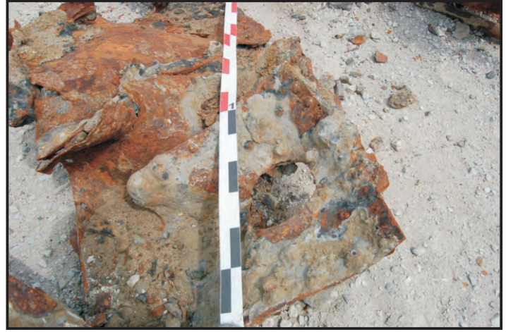
Figures 53 - 54: Internal and external view of porthole, note the strengthening plate on the external side (Photos: Maitland)
