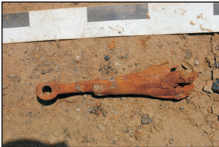
Figures 130 - 131: The opposing ends of a turnbuckle, the first is a fixed eye on the end of a screw and the second is a shackle on the end of a screw. These were used to adjust the tension or length of rigging wires (Manual of Seamanship 1951; Photo: Maitland)
