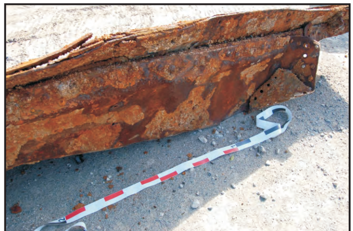
Figure 34: Close-up of the gunwale, where the sheerstrake, bulwark and deck intersect (Photo: Maitland)
