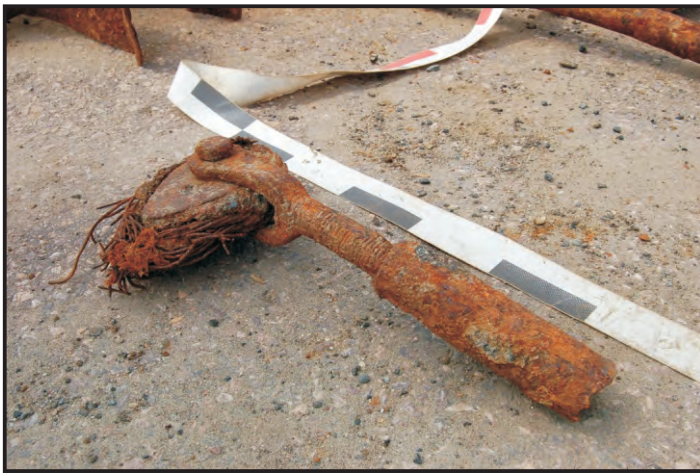
Figure 122: Turning-in screw with thimble, these are used to break in a wire rope (Manual of Seamanship 1951: 147; Photo: Maitland)
