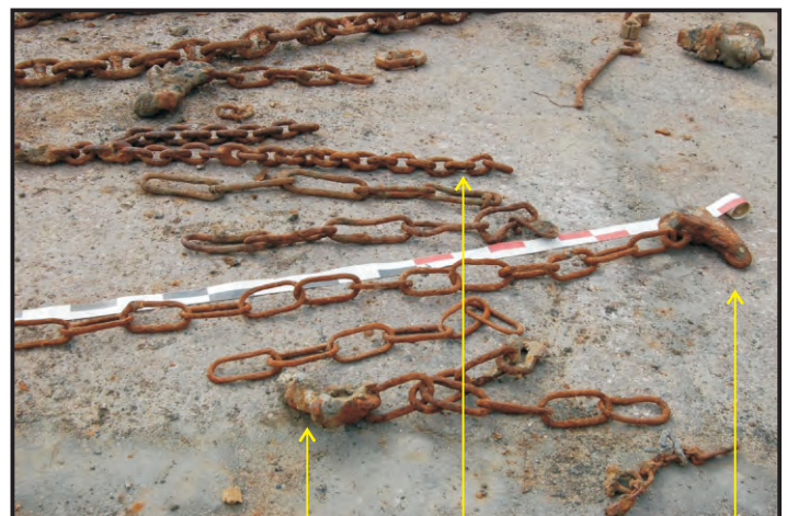
Figure 139: Stud-link, common straight link and open link chains of various sizes and gauges (Carpenter 1917: 600; Manual of Seamanship 1951: 147; Photo: Maitland)
