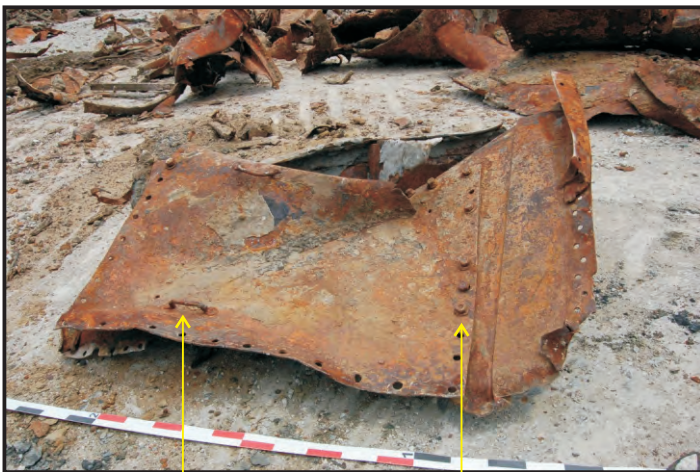
Figures 49 - 50: Front and back of an access hatchway, these were placed throughout the vessel. This has two handles and was bolted shut (Photo: Maitland)
