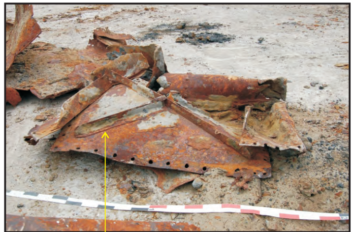
Figures 49 - 50: Front and back of an access hatchway, these were placed throughout the vessel. This has two handles and was bolted shut (Photo: Maitland)
