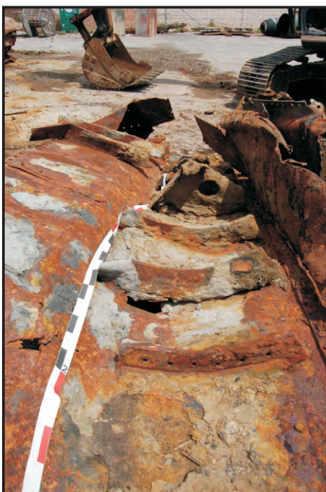
Figures 69 - 70: Two views of the keel, probably forward of midships, these frames are at the turn of the bilge, also bracket frames are visible (Photos: Maitland)
