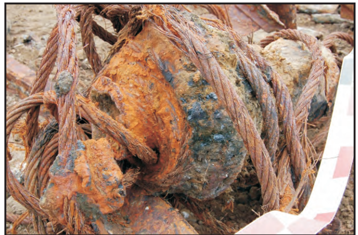
Figures 99 - 100: Steam windlass. According to the Lloyd's Survey of 1921, the Karin had a steam windlass. This was usually placed on the upper fore-castle deck and was used for hauling up bower anchors (Appendix A: 3; Paasch 1890: 156; Photos: Maitland)
