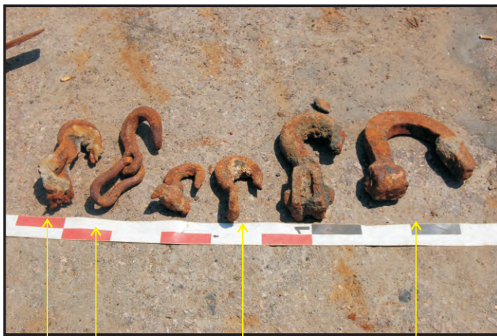
Hooks broken off from blocks Hook with link Hook with thimble Unknown Figure 128: Selection of hooks (Photo: Maitland)
