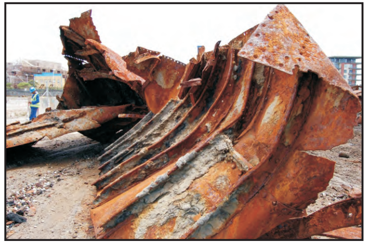
Figure 30: Close-up of the hull plating and the turn of the bilge (Photo: Maitland)
