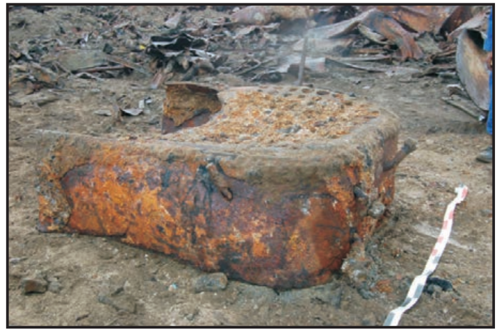
Figures 205 - 206: Views of internal structure of the condenser, the condenser tubes probably fitted through the holes (Photos: Maitland)
