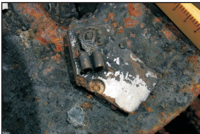
Figure 227: Ceramic electrical connector (Photo: Maitland)
