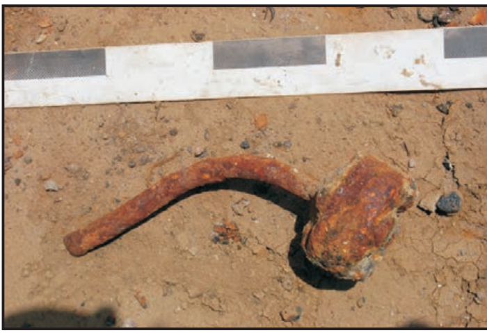
Figure 254: Engineer's hammer (Carpenter 1917: 18; Photo: Maitland)
