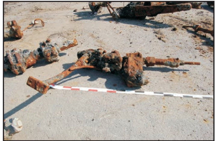
Figures 213 - 214: Views of a crankshaft lubricating oil pump assembly (Renda 2010; Photos: Maitland)
