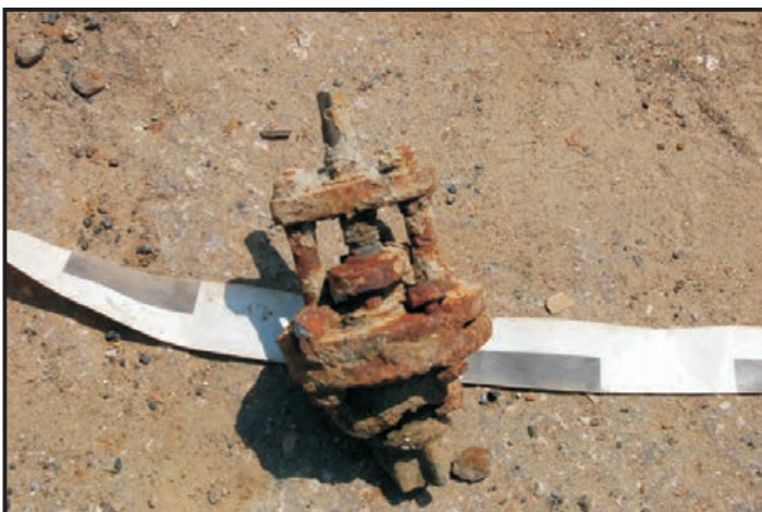
Figure 188: Double-seated valve (Bauer 1905: 141; Photo: Maitland)
