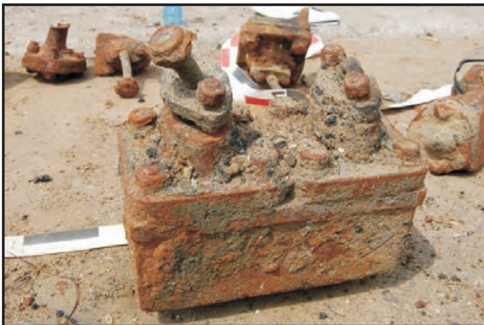
Figure 182: Double stuffing box gland (Photo: Maitland)
