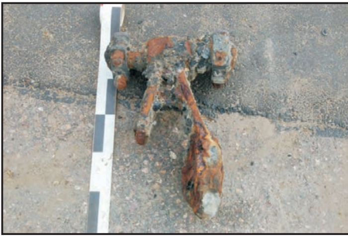
Figure 172: Part of a connecting rod, note the stuffing box glands on either side (Photo: Maitland)
