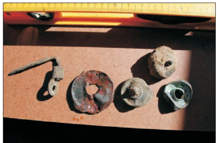
Figure 226: Electric connector, various female nipples and covers for receptacles and rosettes. The second item from the left is stamped — W. Roazs Patent London (Canadian General Electric 1920: 110; Photo: Maitland)
