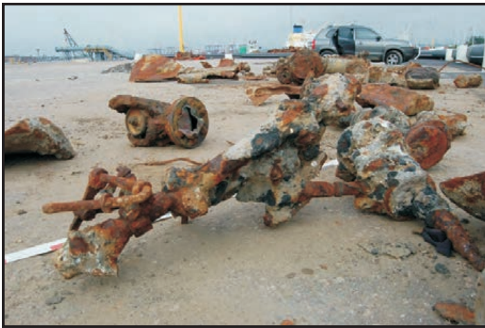
Figures 174 - 175: Two views of connecting rods from the triple expansion engine, the high level of concretion makes identification difficult (Photos: Maitland)
