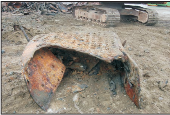
Figures 205 - 206: Views of internal structure of the condenser, the condenser tubes probably fitted through the holes (Photos: Maitland)
