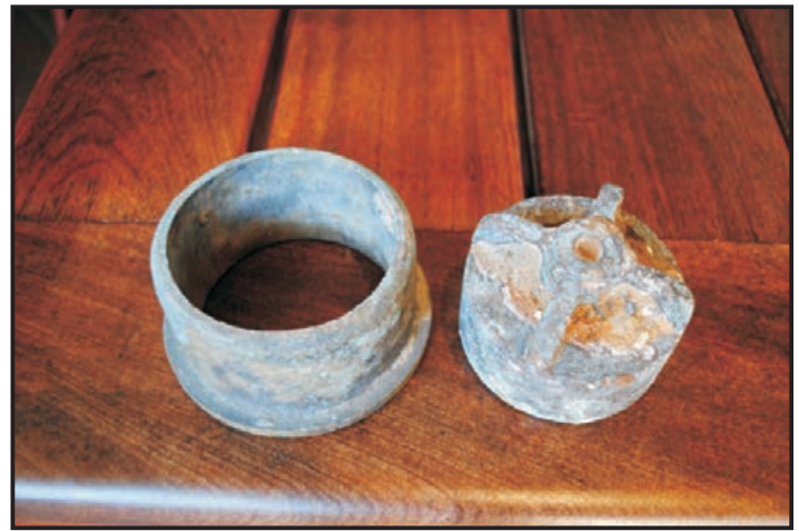
Figure 191: Inner and outer valve parts (Renda 2010; Photo: Maitland)
