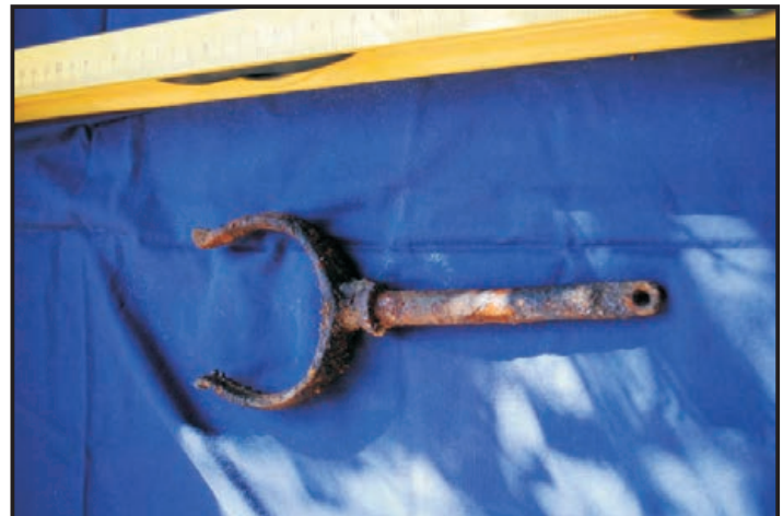
Figure 246: Standard socket rowlock, probably from the Karin's lifeboat (Carpenter 1917: 988; Photo: Maitland)
