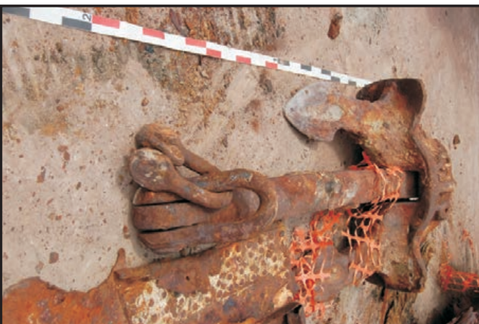
Figure 342: Stockless bower anchor (Paasch 1890: Plate 64; Photo: Maitland)
