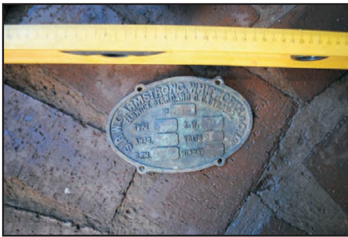
Figure 223: Dynamo's manufacturer's plate — Sir W.G. Armstrong, Whitworth, & Co Ltd. Elswick Standard D.C. Dynamo.
