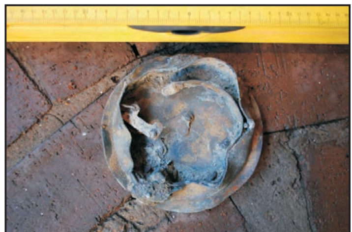
Figure 201: The remains of a Bourbon steam pressure gauge (Morrison 1895:113; Photo: Maitland)
