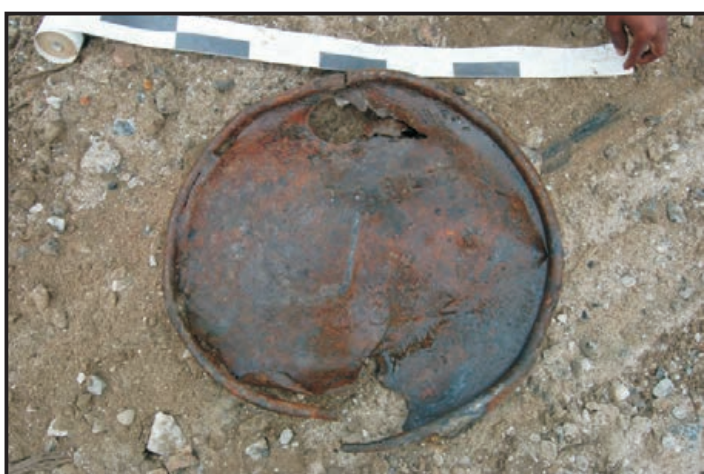
Figure 332: Drum lid with cap missing (Photo: Maitland)
