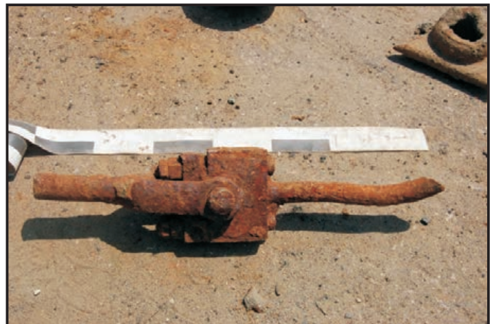
Figure 171: High / intermediate / low pressure connecting rod (Photo: Maitland)
