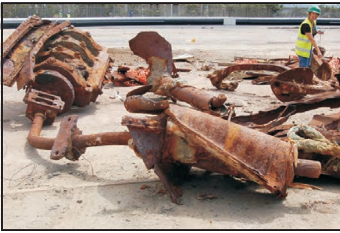
Figure 338: Tunnel shaft bearing and thrust shaft of the propeller (Paasch 1890: Plate 59; Photo: Maitland)
