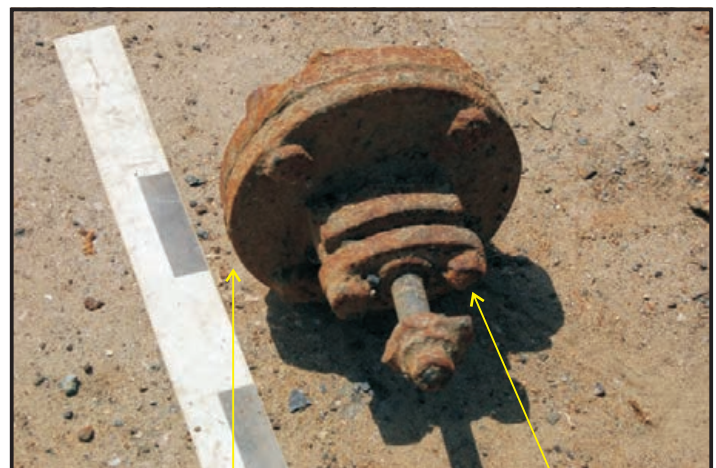
Figure 181: Connecting flange with a stuffing box gland (Photo: Maitland)
