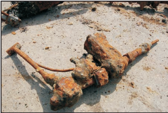
Figures 213 - 214: Views of a crankshaft lubricating oil pump assembly (Renda 2010; Photos: Maitland)
