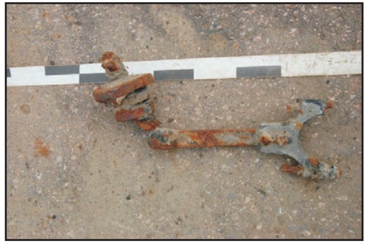
Figure 173: Part of a connecting rod, possibly from an eccentric gear (Photo: Maitland)
