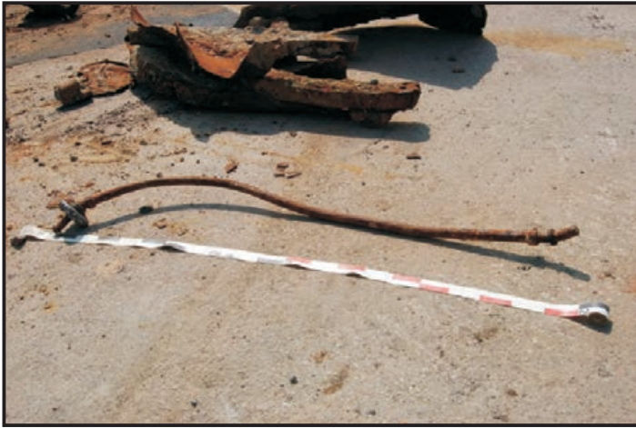
Figure 217: Mitre wheel on a shaft, possibly part of the steering gear (Photo: Maitland)
