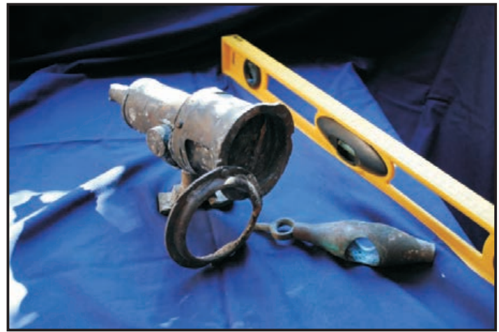
Figure 244: The Karin's taffrail log and governor. The plate is engraved with — Walker's Cherub Ship Log T.W. (Mark II) 900.
