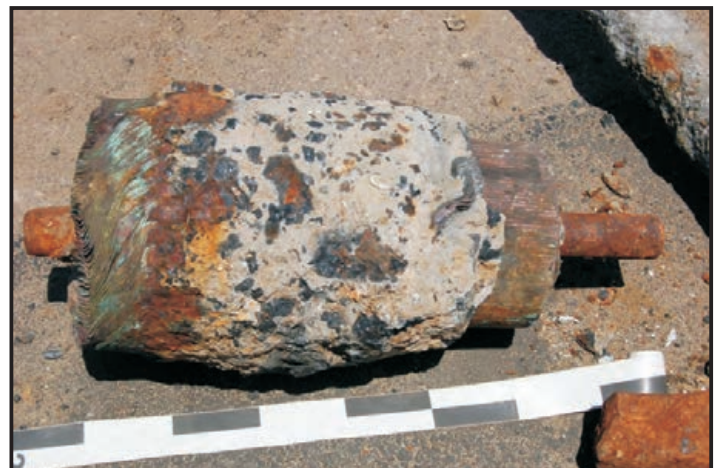
Figure 222: Electric motor armature (Renda 2010; Photo: Maitland)
