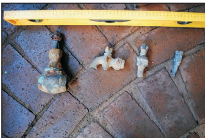
Figure 200: Globe valve, drip tap valve and stop cocks (Photo: Maitland)
