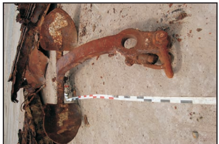
Figure 343: Stockless bower anchor (Paasch 1890: Plate 64; Photo: Maitland)
