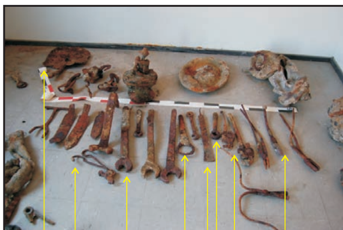
Coal shovel Iron work skidding tongs Chisel scraper Ring spanner Engineer's wrenches Square head wrench for cocks Blacksmith's tongs Monkey wrenches
