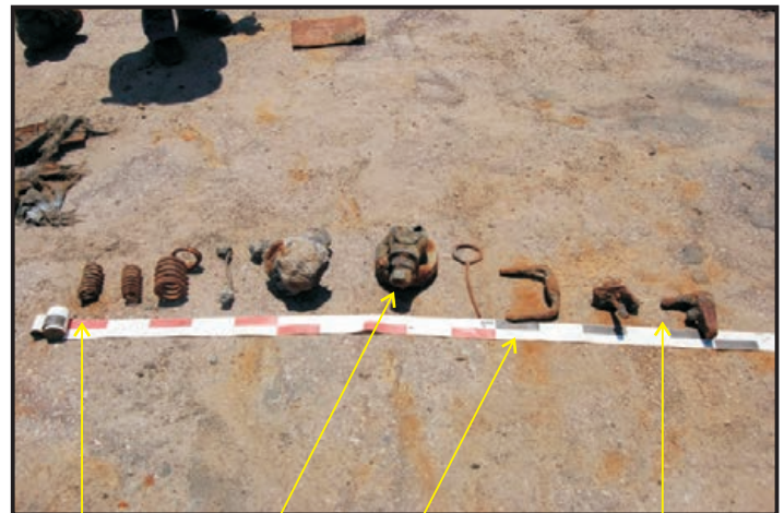
Figure 195: Assortment of miscellaneous equipment (Photo: Maitland) Springs Ball valve Valve handle Stuffing box glands
