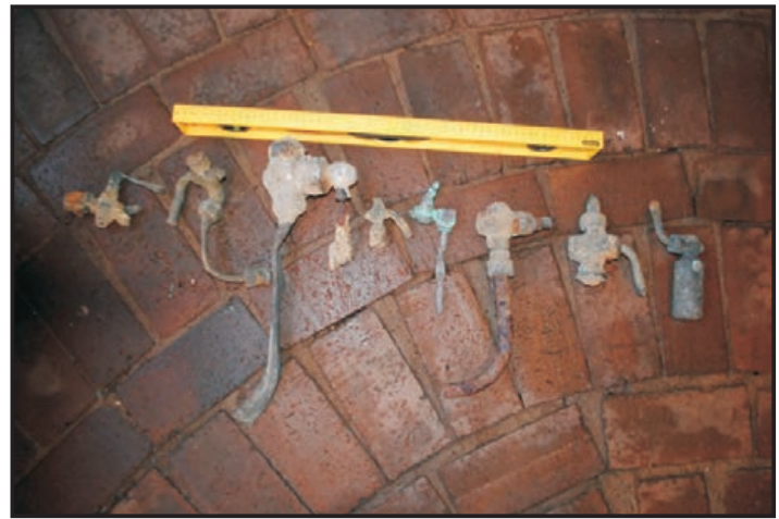
Figure 185: Assortment of ball valves, throttle valves and stop cocks (Photo: Maitland)
