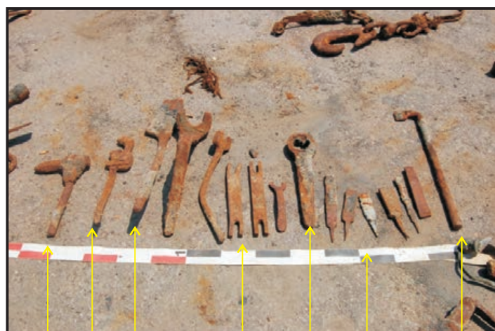
Deck punch Stilson wrench Blacksmith's sledge Open end spanners Flogging spanner Rat tail files Tamping bar
