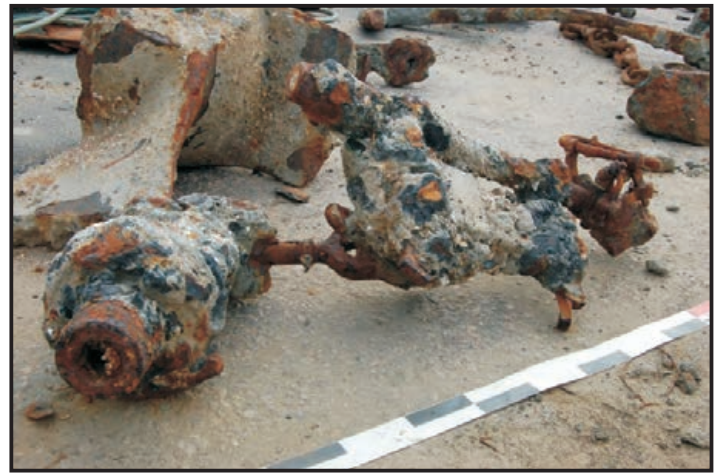
Figures 174 - 175: Two views of connecting rods from the triple expansion engine, the high level of concretion makes identification difficult (Photos: Maitland)
