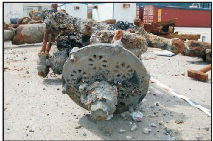
Figures 207 - 208: Views of the main section of bilge pump (Paasch 1890: Plate 53; Bauer 1905: 321; Photos: Maitland)
