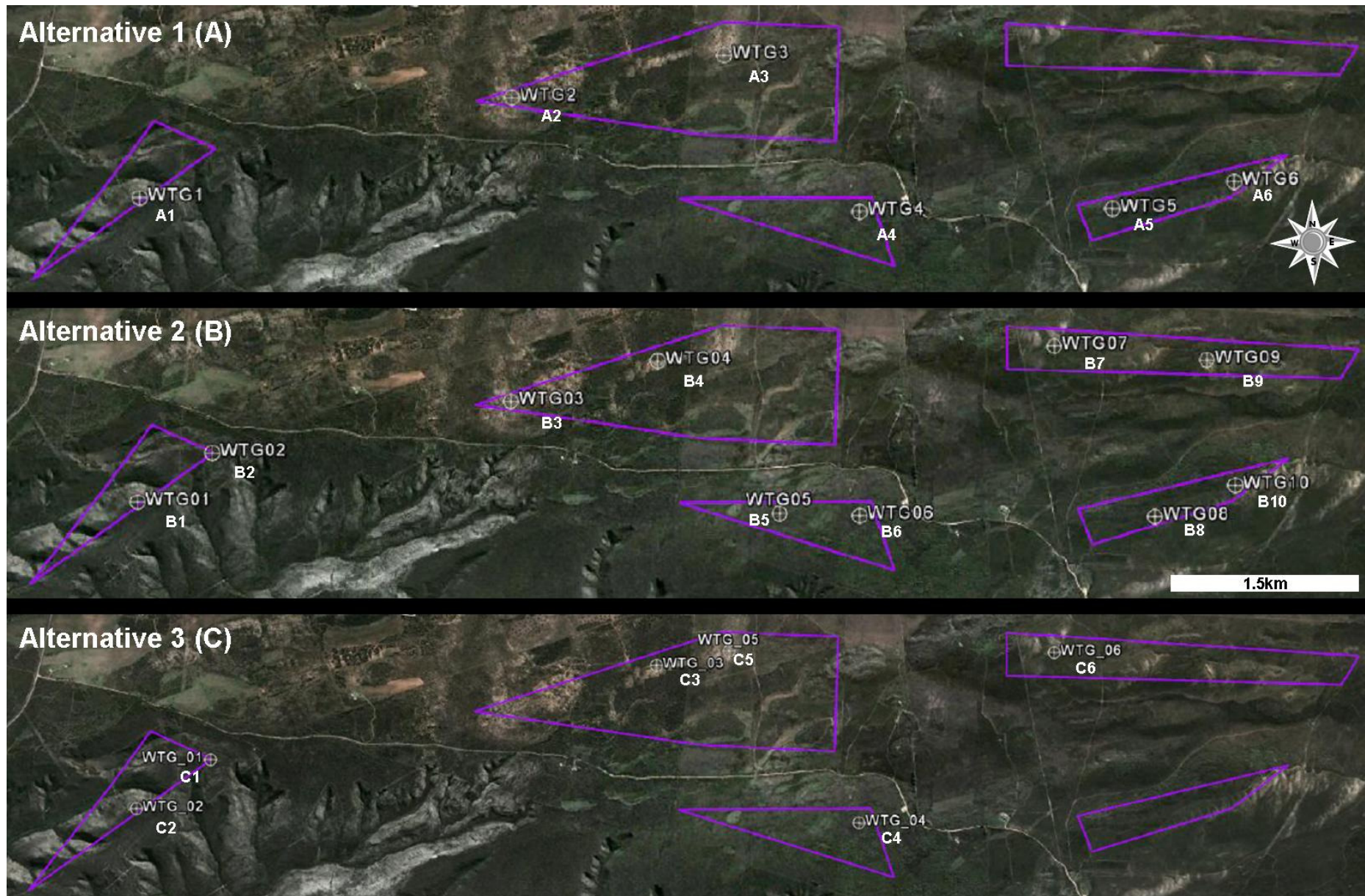
Figure 3. Three alternative layouts for wind turbine placement (courtesy of Cape Environmental Assessment Practitioners (Pty) Ltd).
