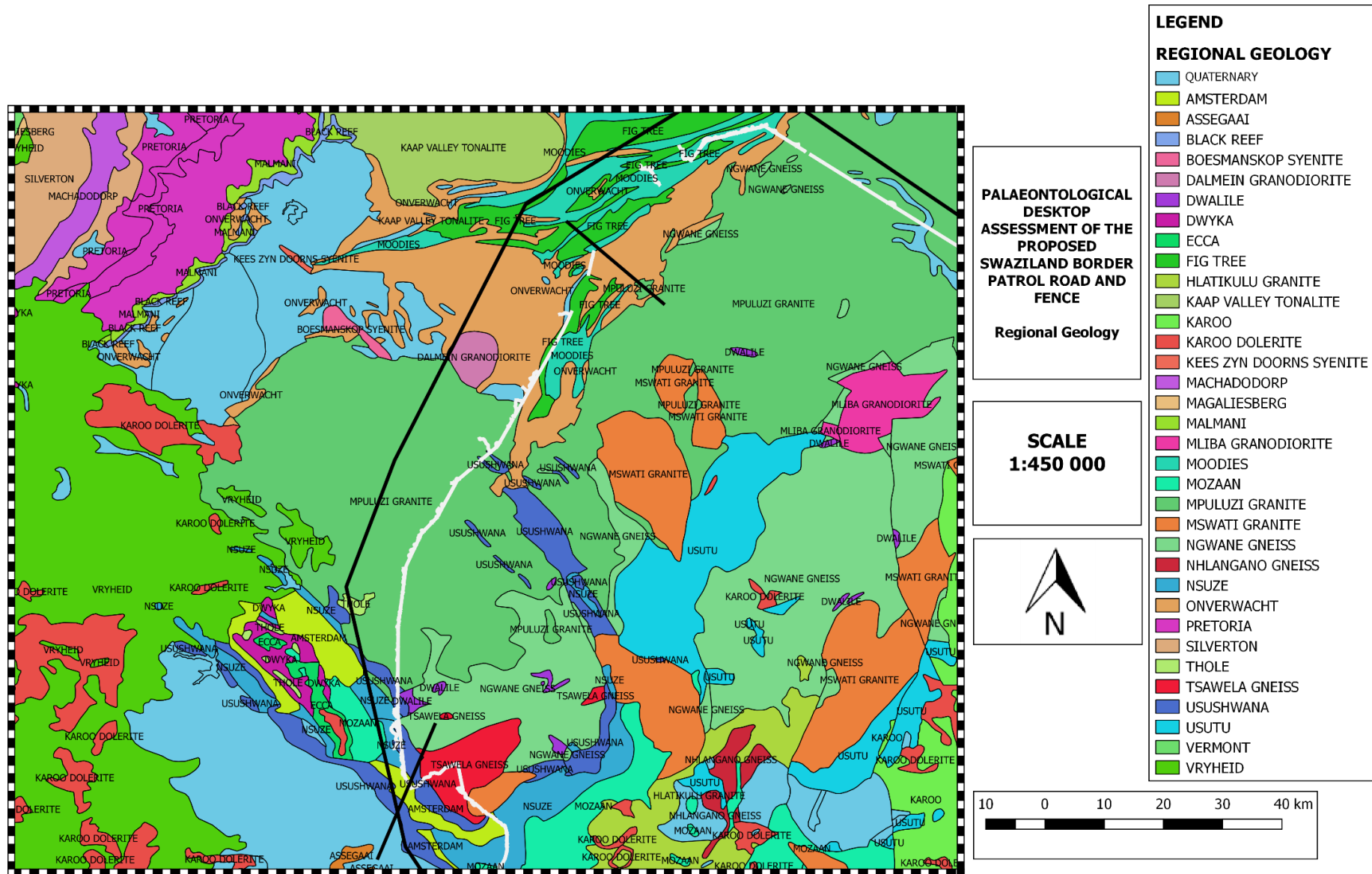
Figure 11: The surface geology of Section F of the proposed Swaziland Border Patrol Road and fence. The proposed development area is completely underlain by Quaternary, Barberton Sequence, Usushwana and Nsuzé Fm. Map drawn QGIS Desktop-version 2.14.20 with GRASS 7.2.2
