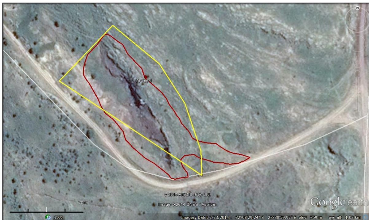
Figure 22. Close-up aerial view of the area proposed for Borrow Pit 186 (BP186) showing the extent of the proposed borrow pit and area surveyed.
